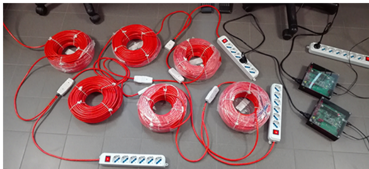
Figure 2.5: Real deployment of an electrical line composed by different pieces of electrical cable.
