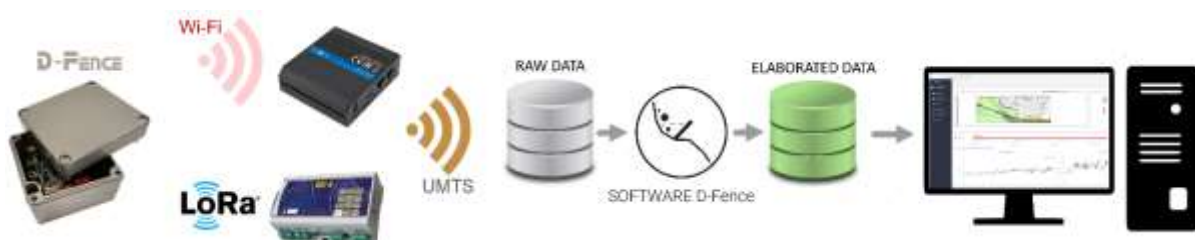
Figure 1. Structure of the D-Fence monitoring system.
