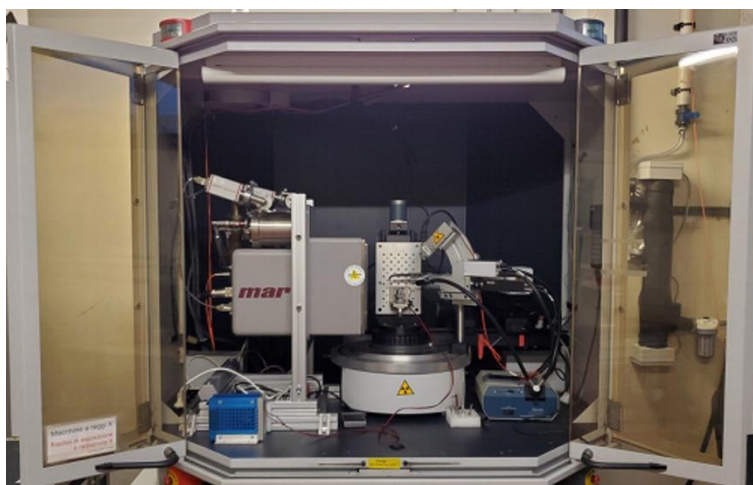
Figure 3.5.2: D8 Advance Bruker diffractometer in a Debye-Scherrer geometry. On the left: 2D detector MARCCD.
