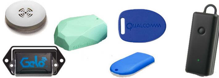
Figure 1.8: Examples of BLE beacons suitable for indoor positioning.
