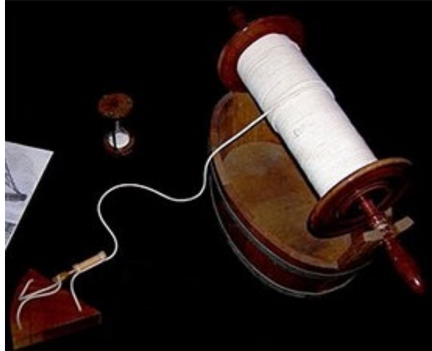
Figure 1.4: A chip log, also called ship log, used to estimate the speed of the ship in knots .
