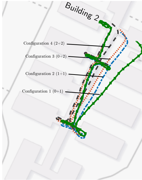
Figure 3.3: Path estimates based on the four different configurations introduced in Section 3.1. The experimental data have been collected during a single walk for a fair comparison.
