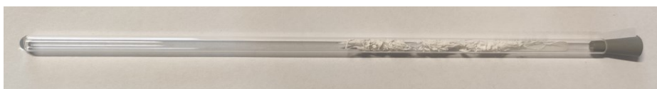
Figure 4.2 – Polymeric fibers composed of PBPMLG into an NMR tube before solvent addition.
