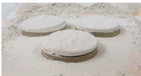
Figure 4.5 Picture of samples before the thermal treatments of debinding and sintering.
