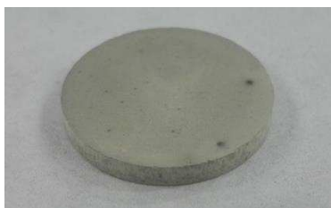
Figure 1.16 Picture of the BCZY-GDC pellet sintered with ZnO as sintering aid at 1400°C for four hours.
