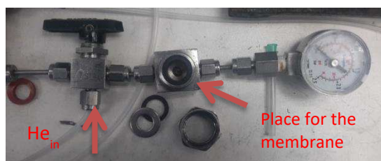
Figure 4.18 Apparatus for the gas-tightness test.
