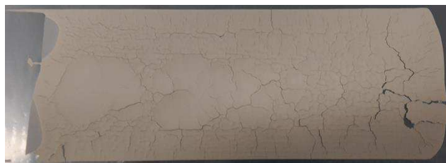
Figure 2.3 Picture of the BCZY_45 tape after drying.
