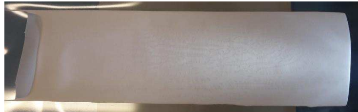
Figure 2.2 Picture of the BCZY_15 tape after drying.
