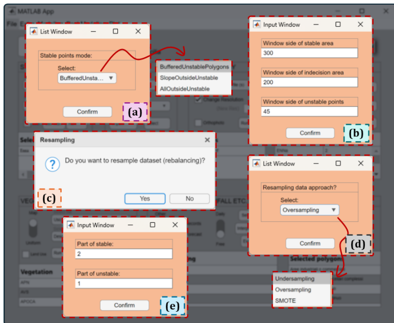
Figure IV-45: Part II of the possible options for the construction of PIP-AI dataset, during the processing of the <Dataset Creation> button (with <Dataset for PIP-AI> flagged). It is possible to select the type of stable area (a); select the buffer sizes for the stable areas (b); decide to resample the dataset (c); select the type of resampling (d) and the ratio between stable and unstable pixels (e), if the user decides to continue with the resampling.
