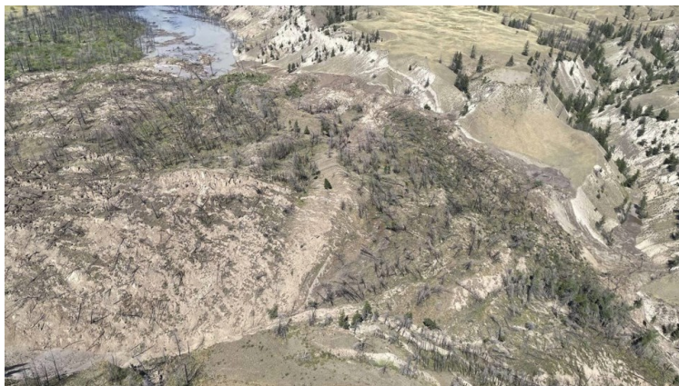
Figure II-6: A combination of shallow landslides and debris flows near the Williams Lake, during the recent flood of July 2024, in British Columbia. The landslide, triggered by rainfall in a deforested area, dammed the Chilcotin River.
