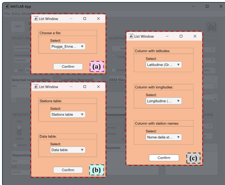
Figure IV-21: The “matching” prompts for the time sensitive panel, which appear after pressing the <Select file (s)> button. It is possible to select the file to use (a). If the file is a spreadsheet, it is necessary to specify the match between the various tabs of the file and the ‘Data table’ and ‘Station table’ ones (b). Similarly, if the file is a spreadsheet, it is also necessary to match the three main columns of the ‘Station table’, containing the names of the gauges and their geographic coordinates (c).
