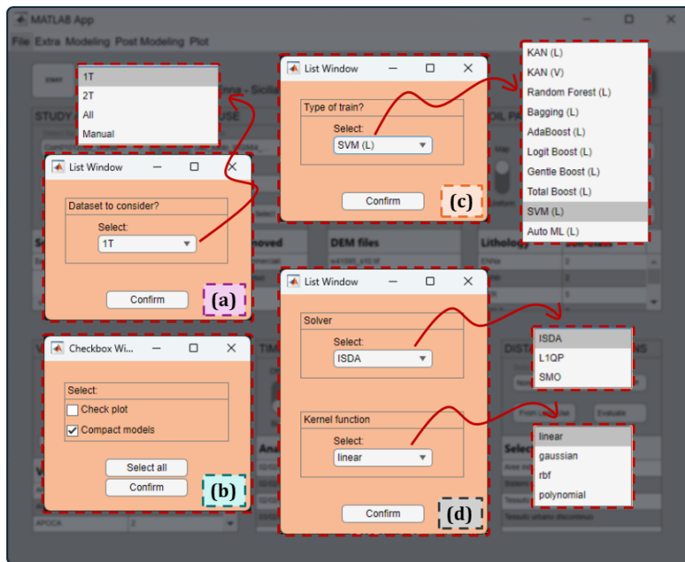
Figure IV-55: Part I of the possible options during the process triggered by the <PIP-AI (Generic)> button, inside the "Machine Learning" group of the "Modelling" top-menu. It is possible to select what are the datetimes to use from the general dataset (a); select if the models must be stored as compact and to create a fast 'check' plot (b); select the type of machine learning model and training (c); specify some of the main hyperparameters for the Support Vector Machines (if <SVM (L)> was selected) (d).
