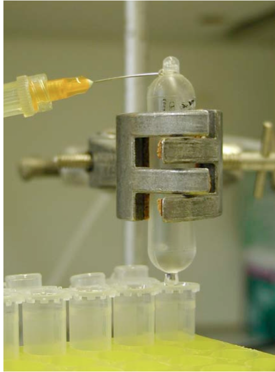
Fig. 6 Fractionation of SIP ultracentrifugation gradients via a syringe pump and manual fraction collection.
