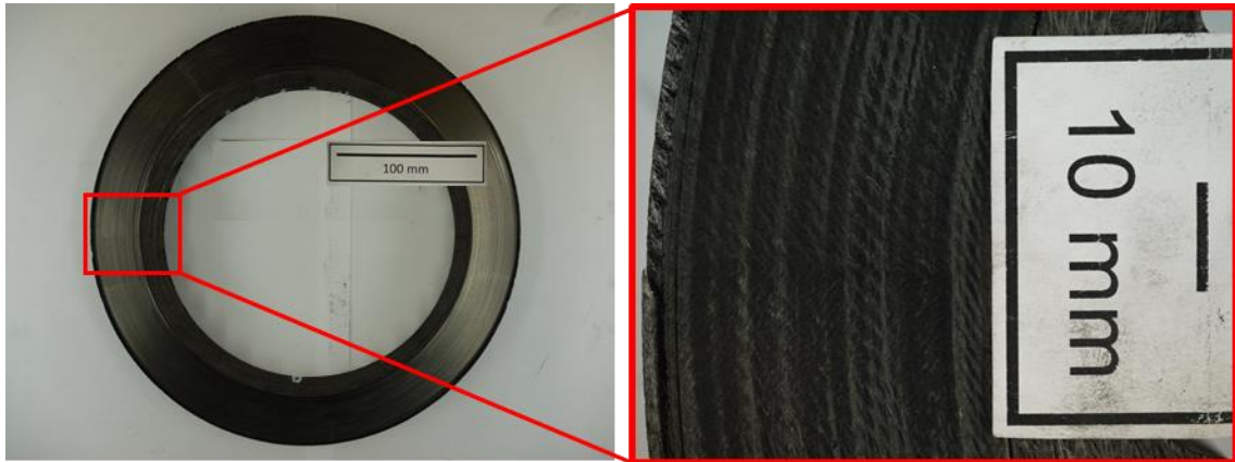
Fig. 7.19: C/C-Disc after braking test with ZL material at 1 MPa.
