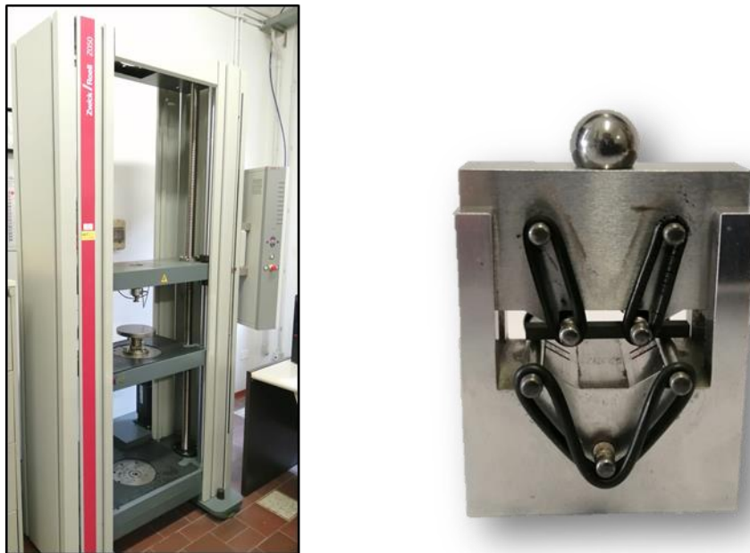
Fig. 3.8: Four-point geometry reported in ISO 14704:2016 and relative formula for the flexural strength calculation. Where, P_N is the force in newton, P_{Kg} is the force in Kg and b and d are the width and thickness respectively.
