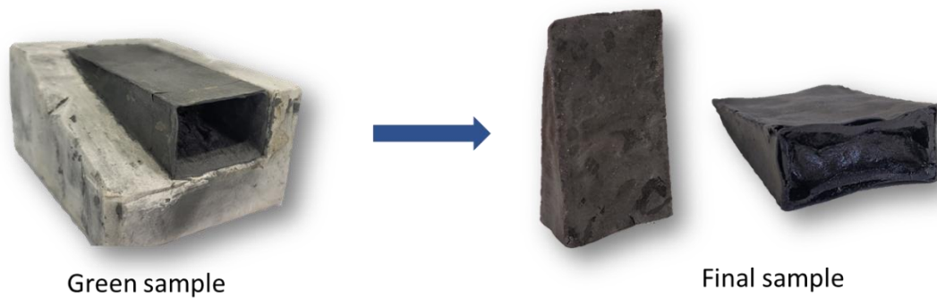
Fig. 6.16: Images of the green sample and of the sample after four cycles of PIP.
