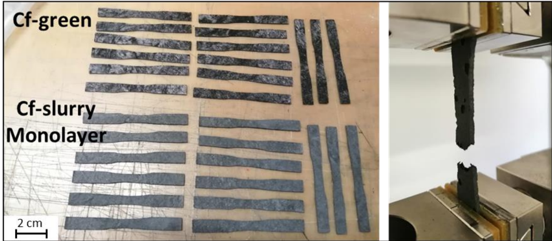
Fig. 4.5: images of the dog-bones Cf-Green and Monolayer (left) and a dog-bones during the test (right).
