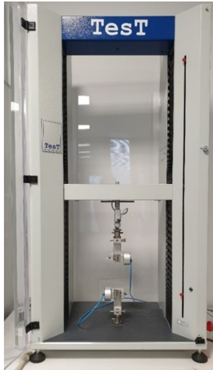
Figure 2.10 - Test dynamometer used for uniaxial tensile testing (UTT)
