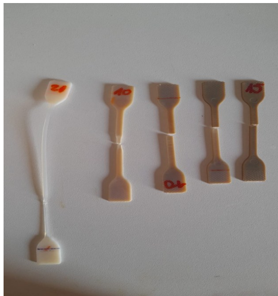
Figure 2.18 - Specimens 5A obtained by injection molding after tensile testing, from left to right: PBAT, PBAT+5%HF, PBAT+10%HF, PBAT+20%HF, PBAT+40%HF
