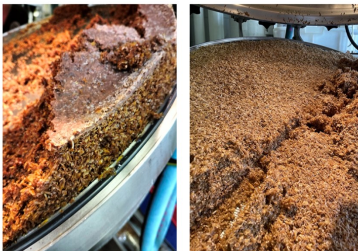
Figure 3.34 - BSG filter cakes after the conventional lautering process with a presence of a gelatinous film (left) and after the alternative lautering process with no visible presence of such film (right)
