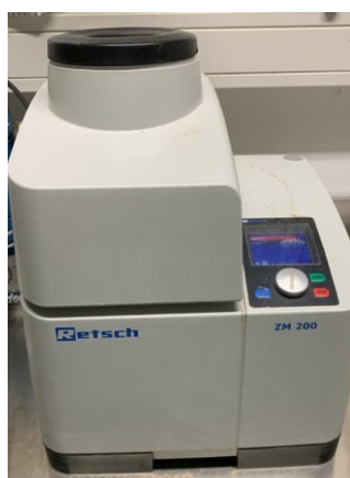
Figure 3.29 - Centrifugal mill ZM200 used for grinding the three different fillers (BSG, S2_T2 and S2_T3)
