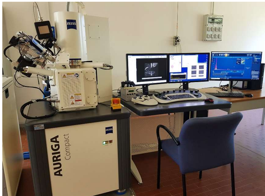
Figure 3.15 – FESEM-FIB with EDS tool at IMEM-CNR
