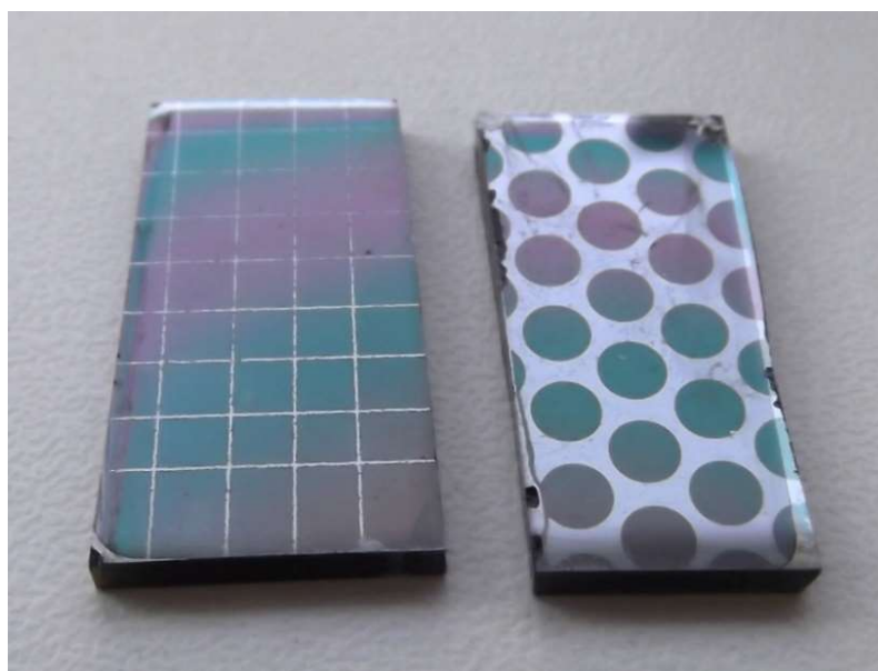
Figure 4.32 – Two halves of the same Sb_2Se_3 -based solar cell, processed in different ways for sub-cells separation: laser-scribing (on the left) and photolithography (on the right)
