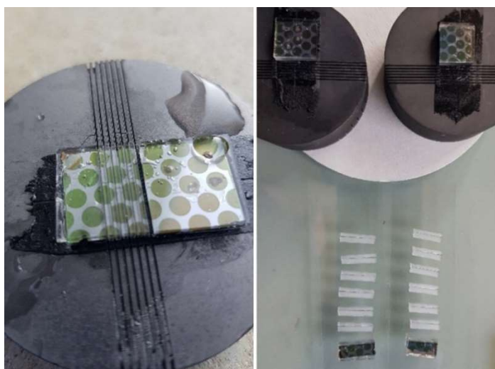
Figure 4.61 – preliminar cut of thin slices from the cells
