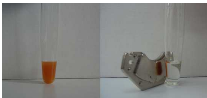
Figure 4.21: Left: Diphenyl \text{Fe}_3\text{O}_4 nanoparticles dispersed in solution, Right: MNPs collection by a magnet
