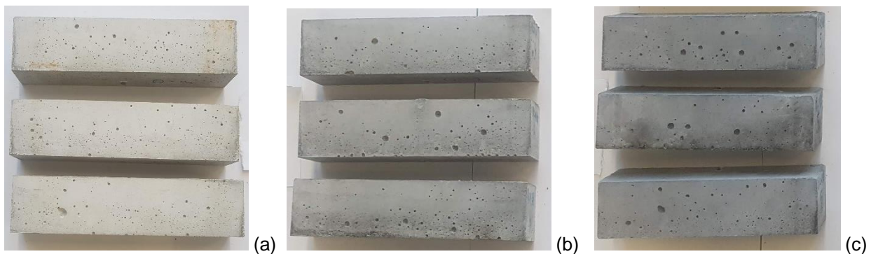
Figure 6 – 40 mm x 40 mm x 160 mm prisms of: (a) REF, (b) BIO2, and (c) BIO5 mixes after 2 years curing.
