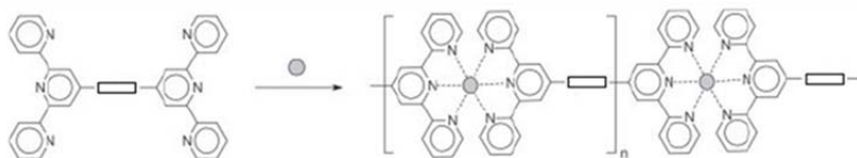
Figure 4.4: Scheme of a terpyridine based supramolecular linear polymer.
