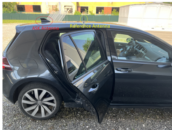
Figure 3.12: Experimental setup: ASK antenna (left) and reference antenna (right).
