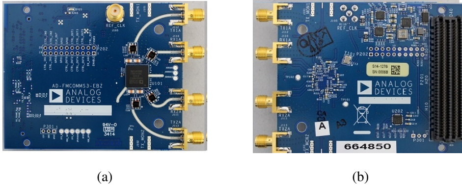
Figure 2.7: Analog Devices AD-FMCOMMS3-EBZ Front End: (a) top view; (b) bottom view.
