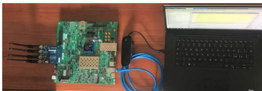
Figure 2.11: Experimental setup with Wireless Loopback model.
