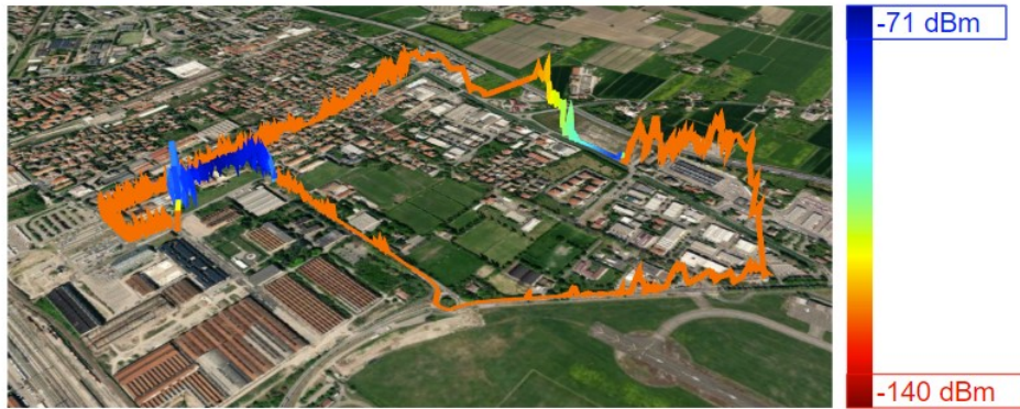
Figure 3.27: A combined presentation of RSRP (color) and DL throughput (line height) using the reference antenna, based on tests conducted across a test path.
