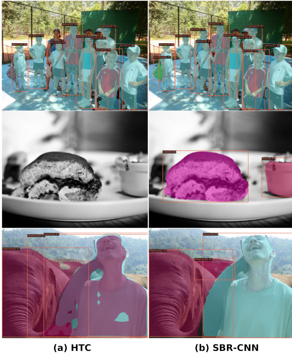
Fig. 7. Examples of instance segmentation comparison between HTC (left) and SBR-CNN (right), filtered with a class confidence threshold of 0.7.
