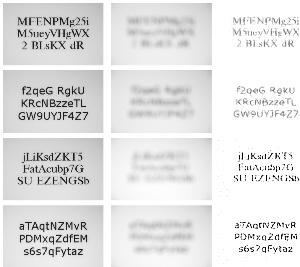
Figure 3.7: From left to right: ground truth, noisy sample and reconstruction using the SVR merit function with K = 70 inner iterations. From top to bottom, two images, one per font, are selected for the steps 10 and 12. The corresponding scores are shown in Table 3.2
