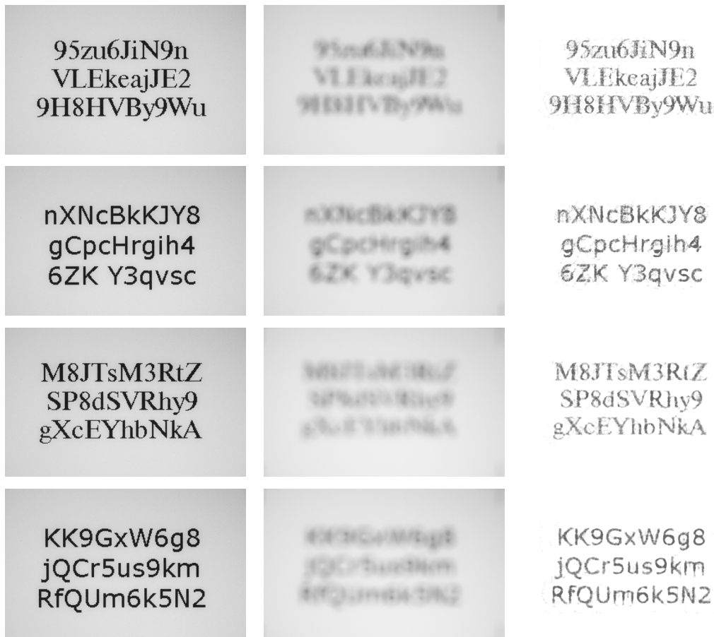
Figure 3.6: From left to right: ground truth, noisy sample and reconstruction using the SVR merit function with K = 70 inner iterations. From top to bottom, two images, one per font, are selected for the steps 6 and 8. The corresponding scores are shown in Table 3.2.
