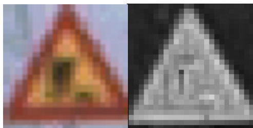
Figure 3.14: Example of sign where the edges of the inner triangle are not well contrasted; on the other hand the border separating the sign from the background is visible.
