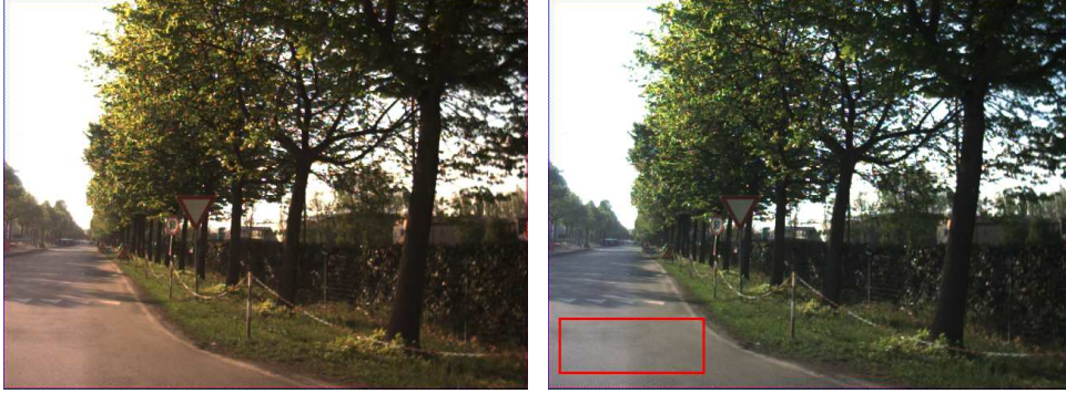
Figure 3.5: Original image and result of chromatic equalization. In the right image the region supposed to frame the pave is shown.
