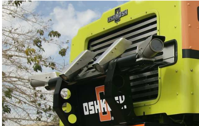
Figure 4.6: The front stereo system mounted on the TerraMax vehicle.
