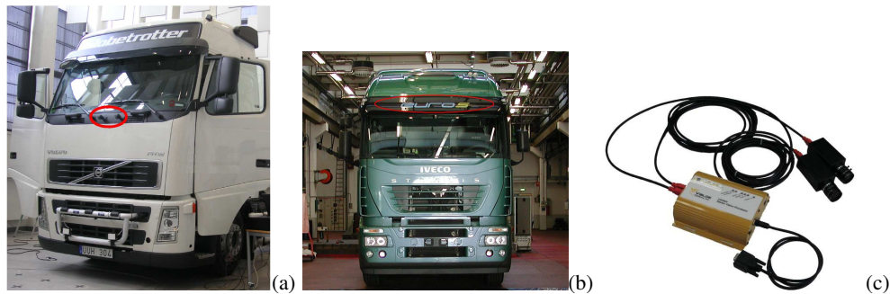
Figure 4.5: Stereobox mounted on (a) Volvo and (b) Iveco trucks: a red circle highlights cameras position. (c) shows VOD, the embedded version of StereoBox.
