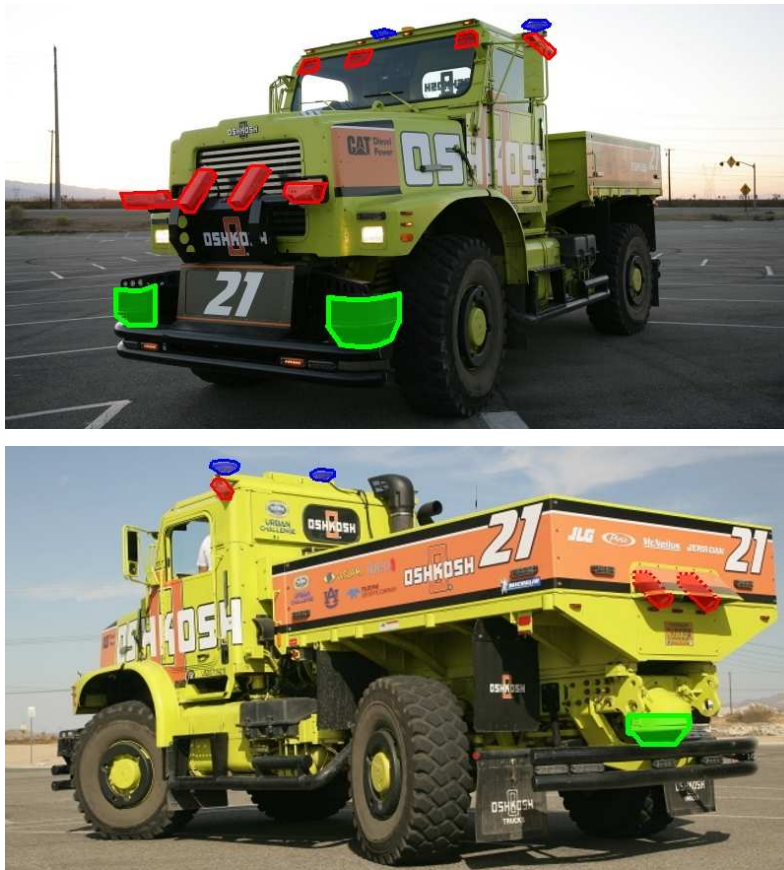
Figure 4.9: All the Terramax sensors highlighted. Color coding: red – cameras; green – laserscanners; blue – GPS antennas.
