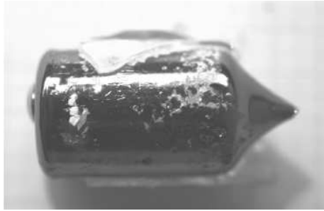
Figure 2.7: A CdZnTe crystal still partially inside the quartz crucible
