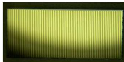
Figure 3 The CZT sensitive unit seen from the anode side that consists of a set of 63 microstrips. The strips are 0.15 mm wide and have a pitch of 0.3 mm.
