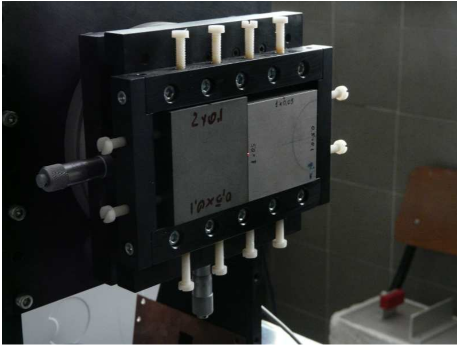
Figure 5.10: Collimator. In figure we can see the laser spot coming out from the slit
