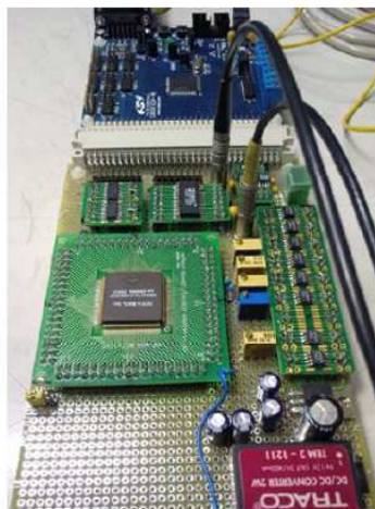
Figure 4. The RENA-3 demo board realized to test the ASIC functionalities before the final readout electronics implementation.
