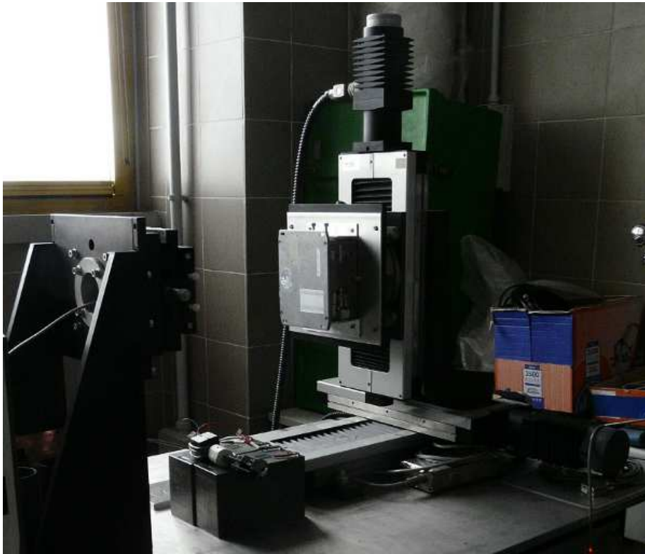
Figure 5.12: System for collimation and centering and the read-out electronic box.
