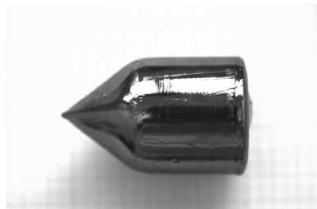
Figure 2.6: 2-inch crystal grown by B_2O_3 encapsulated vertical Bridgman apparatus
