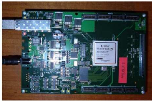
Figure 5. The DHE main board currently under test. The FPGA (a Xilinx VIRTEX 5) core is clearly visible on the right together with the high density connectors to the I/F daughter board.
