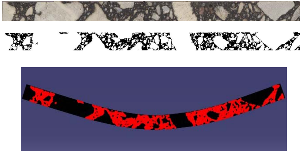
Figure 6.16. Processed image of asphalt mixture beam used as input structure into ABAQUS (red represents mastic and black aggregates)
