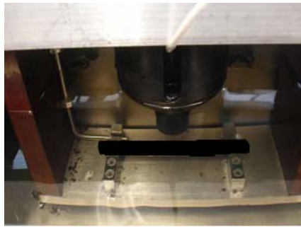
Figure 3.1. BBR equipment for asphalt binder testing
