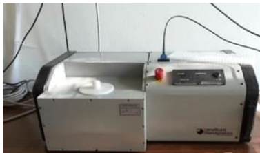
Figure 2.5: DM2 applicator for magnetic hyperthermia (nanoScale Biomagnetics).
