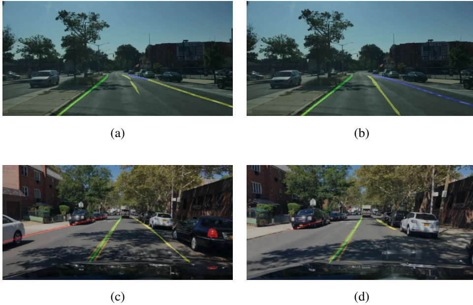
Figure 4.13: Qualitative instance segmentation results for lane detection. Two cases where the network in subsequent frames obtains really different results.
