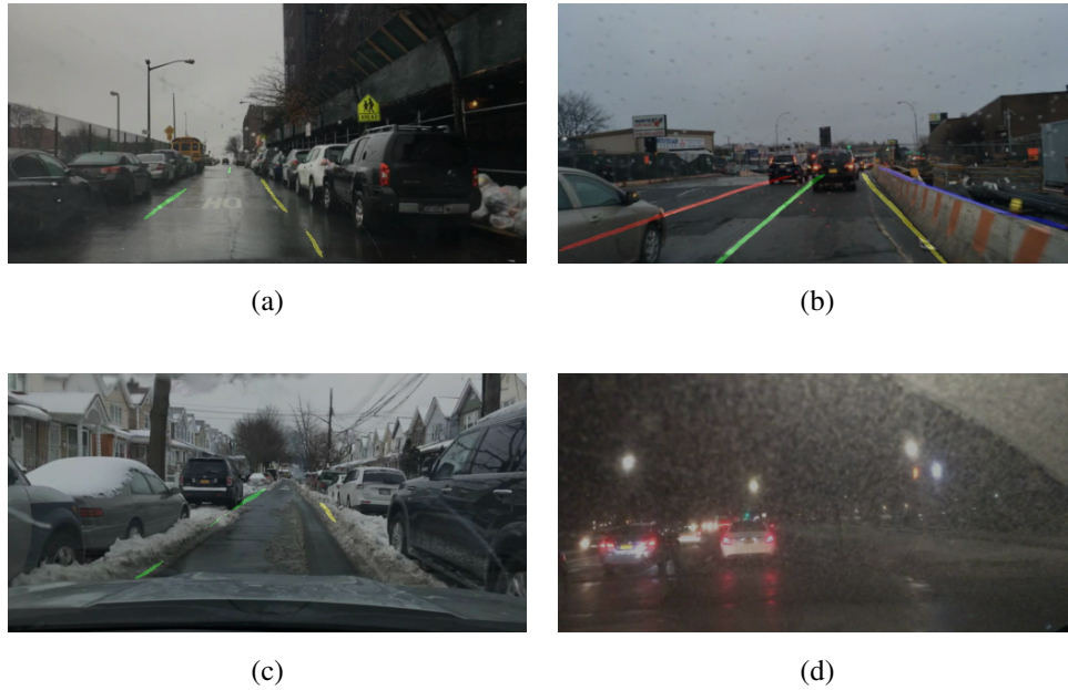
Figure 4.12: Qualitative instance segmentation results for lane detection in case of challenging scenarios where the network fails.
