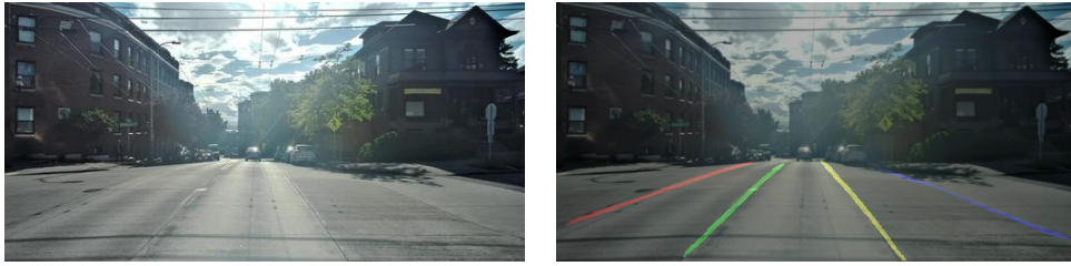
Figure 4.11: Qualitative instance segmentation results for lane detection. On the left column is shown the RGB image and on the right column is shown predicted segmentation over the image.
