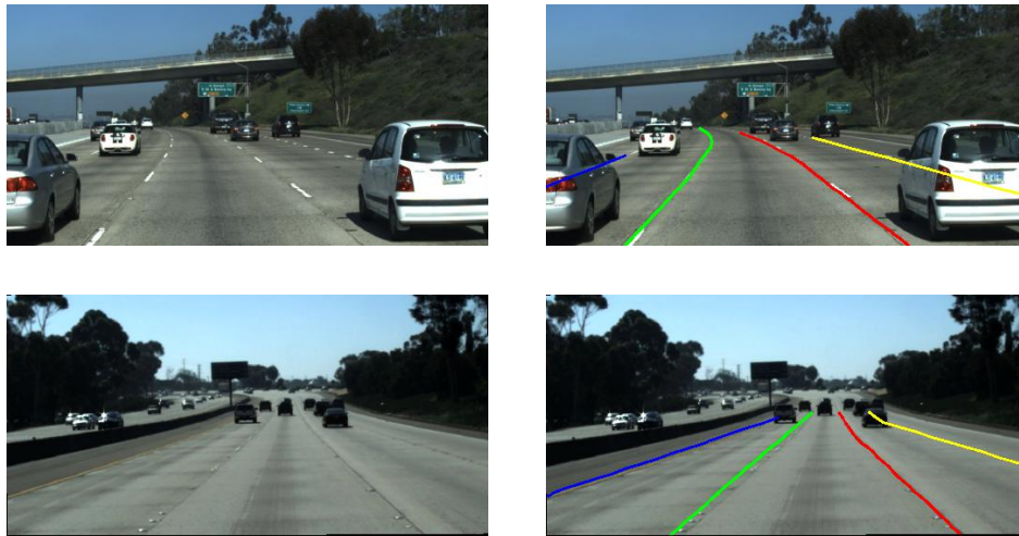
Figure 3.5: Examples of lane detection with all four lanes boundaries: ego lane left (green), ego lane right (red), left lane (blue), right lane (yellow). On the left are displayed the original images while on the right are displayed the annotated images.
