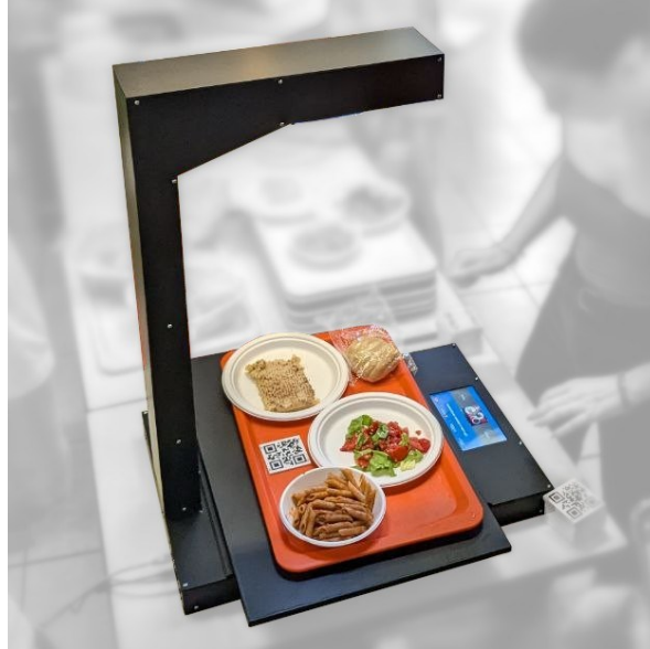
Figure 3. The acquisition device used within the data collection campaign for the FLIC dataset.
