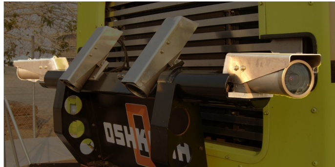
Figura C.2: The two lateral cameras
