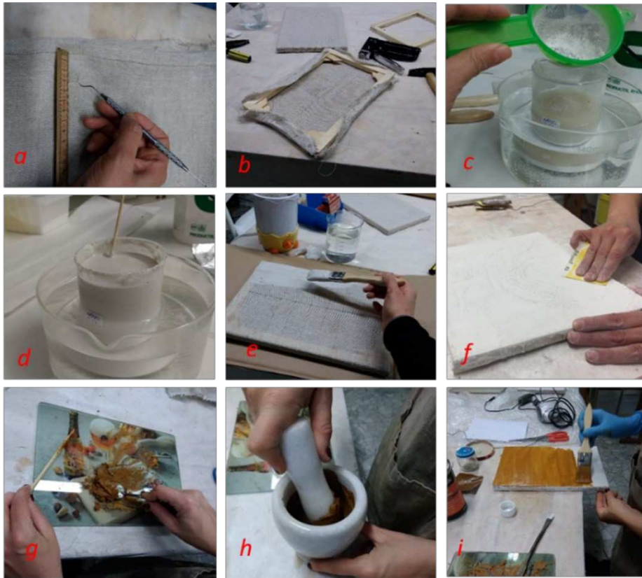
Figure 1- Sample preparation phases: a) evaluation of yarn orientations; b) tensioning on the frame; c-d) plaster and glue preparation; e - f) drafting of the preparatory layer; g-h) preparation of oil color; i) application of the pictorial layer in oil
