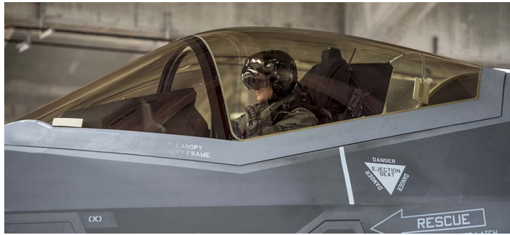
Figure 5: Pilot seated within the cockpit of a modern fighter aircraft featuring a laminated transparency canopy. The canopy consists of multiple polymer–glass laminate layers designed to provide high optical clarity, aerodynamic smoothness, and resistance to impact and thermal gradients. Such aerospace glazing systems exemplify advanced laminated materials where the viscoelastic properties of polymer interlayers play a critical role in ensuring safety, durability, and optical performance under extreme service conditions.
