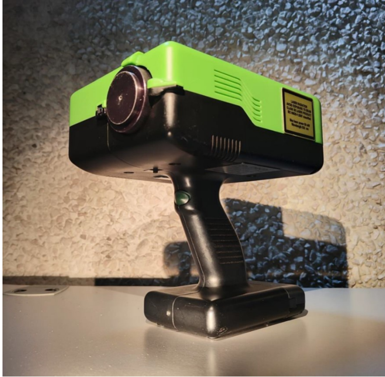
Figure 13: The EnSpectr RaPort handheld Raman spectrometer.
