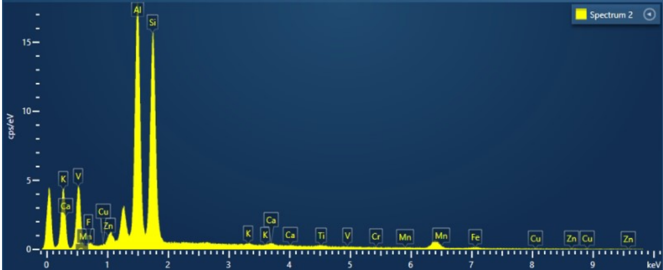
Figure 25: EDS spectrum of sample L2 visualised on AZtecLive® software.
