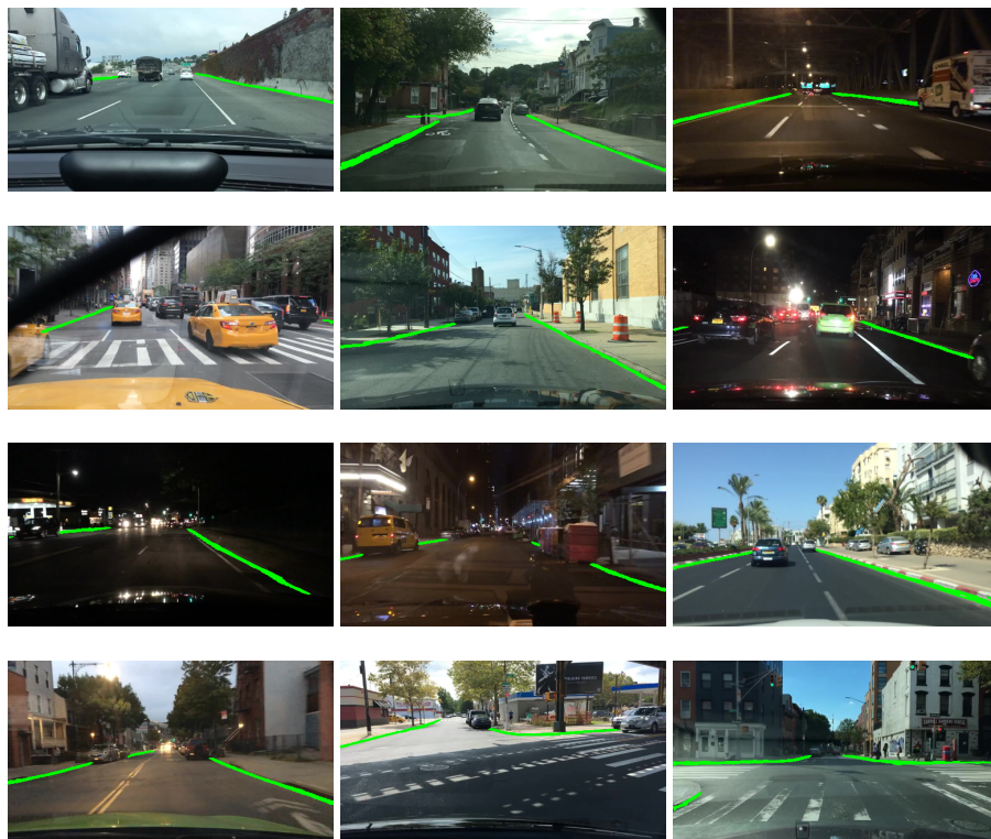
Figure 5.10: Segmentation results examples from BDD100k dataset [1], where curbs are highlighted in green.
