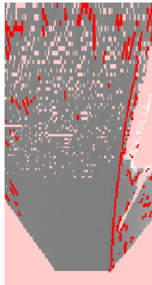
Figure 3.11: Non-maxima suppression result where valid edges are highlighted with red.
