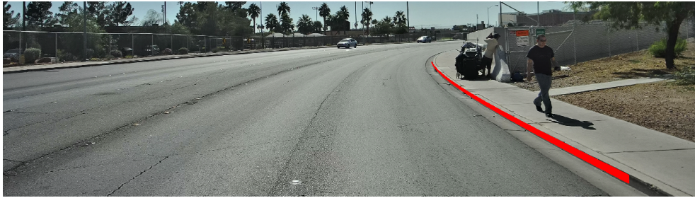
Figure 3.16: Algorithm final result: the detected curb is reprojected back onto the right image
