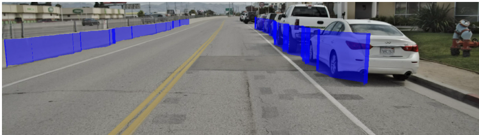
Figure 4.10: Algorithm final result: the detected barriers are reprojected back onto the right image.
