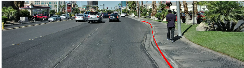
Figure 3.18: Example of curb which cannot be modeled with the chosen polynomial model.
