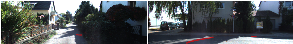
Figure 3.27: Examples of images with false positives curbs caused by shadows and saturation.
