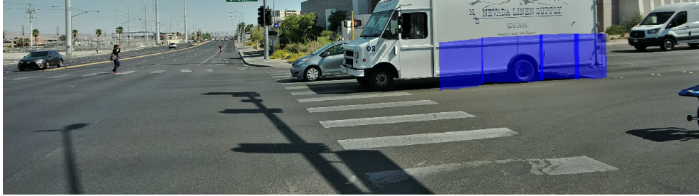
Figure 4.12: Example of a false barrier detected in correspondence of a slowing-moving object.
