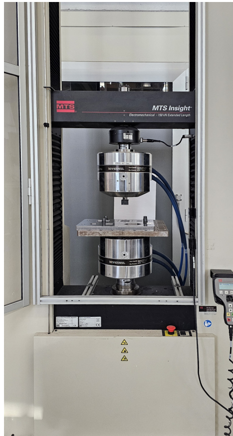
Figure 7.5. MTS Insight 150 kN testing machine with dedicated fixture for penetration tests.
