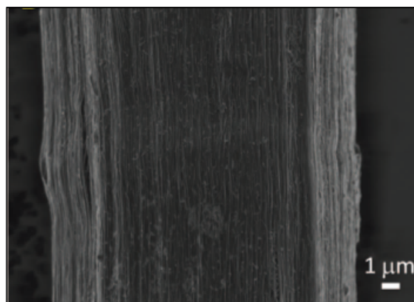
Figure 2.25. Low-magnification SEM image showing the typical morphology of Wet-Spun CNT Fibers [54].
