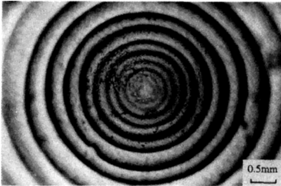
Fig. 2.15 Magnified view of concentric rings within a melt pool in 1100 aluminium alloy [134]
