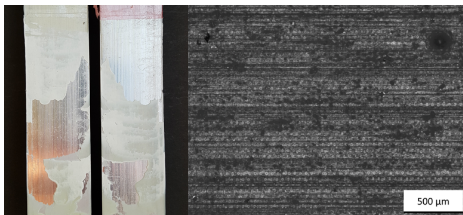
Fig. 5.16 Fracture surface of a C-joint ablated with ED=0.17 \text{ J/mm}^2 and H=50 \mu\text{m} [149]
