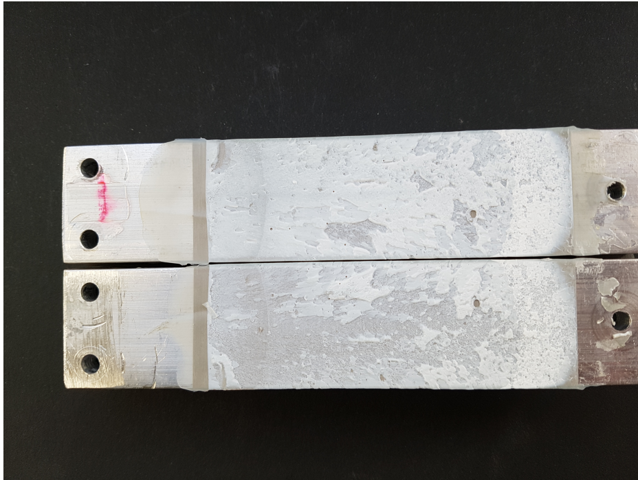
Fig. 5.27 Fracture surface of a fatigue tested T-joint ( ED=0.34 \text{ J/mm}^2 and H=50 \mu\text{m} ) [158]
