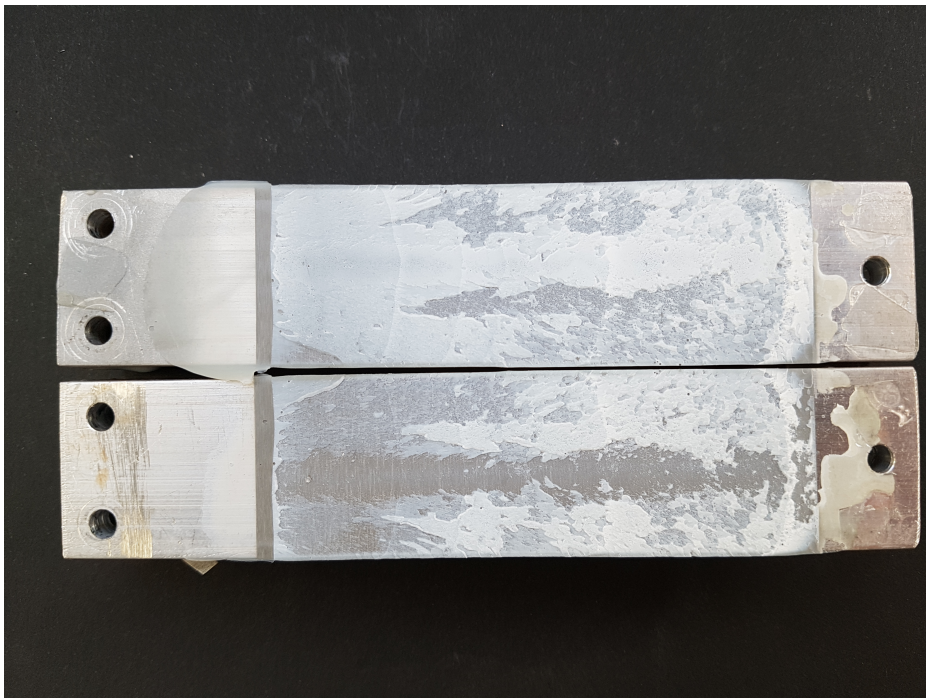
Fig. 5.30 Fracture surface of a fatigue tested T-joint ( ED=1.71 \text{ J/mm}^2 and H=50 \mu\text{m} ) [158]
