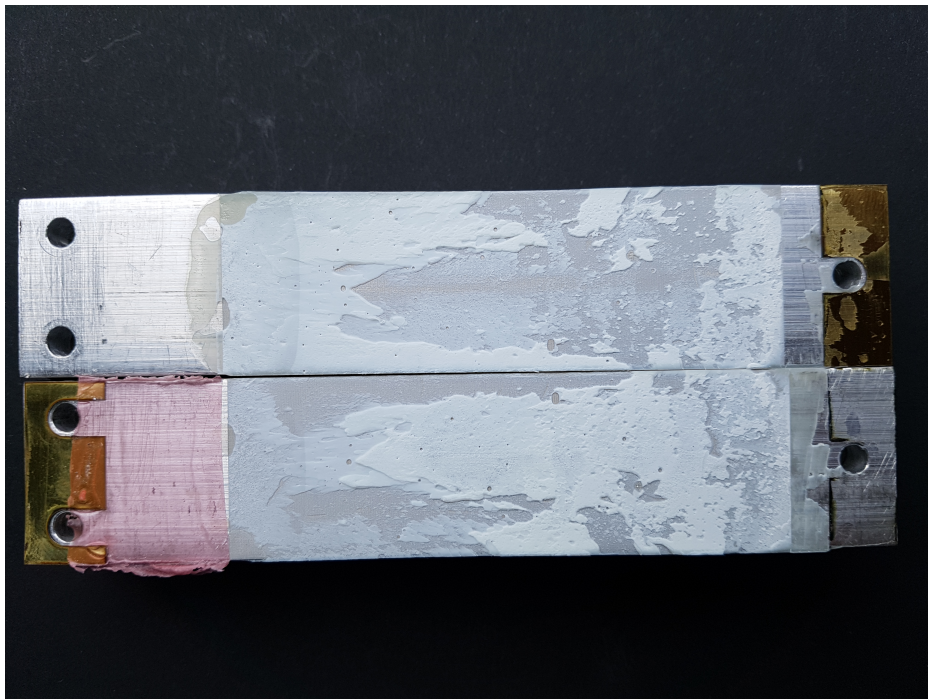
Fig. 5.39 Fracture surface of a fatigue tested C-joint ablated with ED=0.51 \text{ J/mm}^2 and H=100 \mu\text{m} [158]
