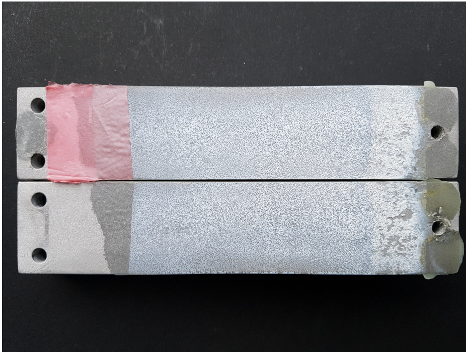
Fig. 5.25 Fracture surface of a fatigue tested grit blasted joint [158]
