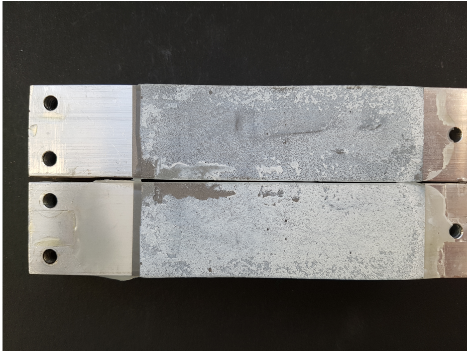
Fig. 5.31 Fracture surface of a fatigue tested T-joint ( ED=3.81 \text{ J/mm}^2 and H=50 \mu\text{m} ) [158]
