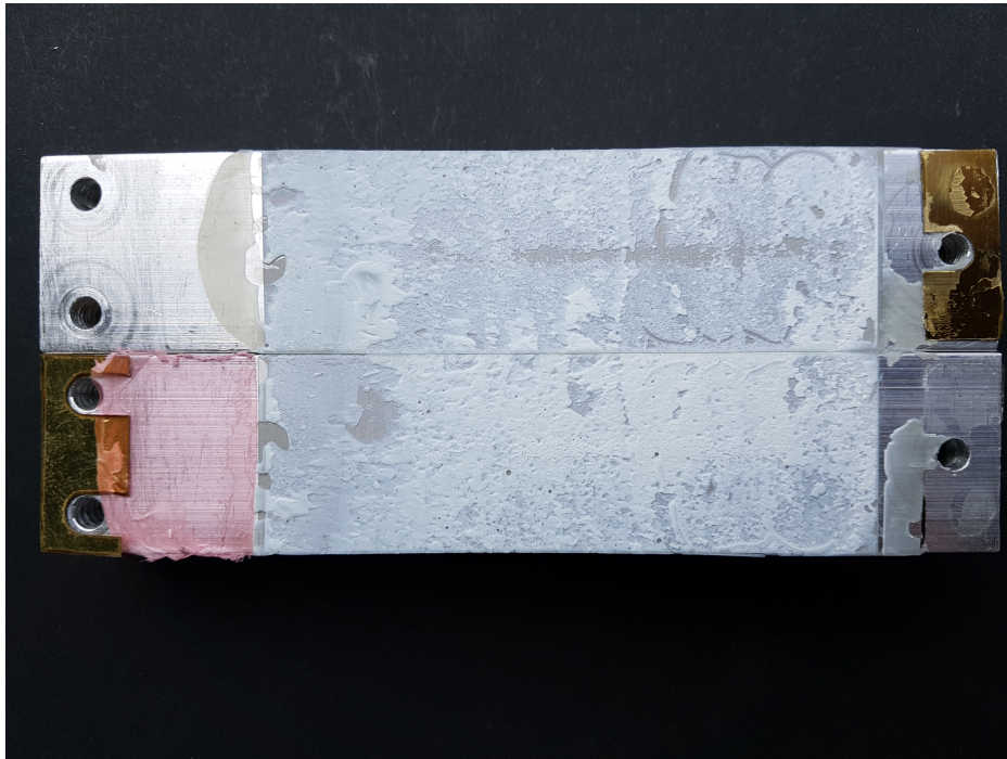
Fig. 5.38 Fracture surface of a fatigue tested C-joint ablated with ED=0.51 \text{ J/mm}^2 and H=50 \mu\text{m} [158]
