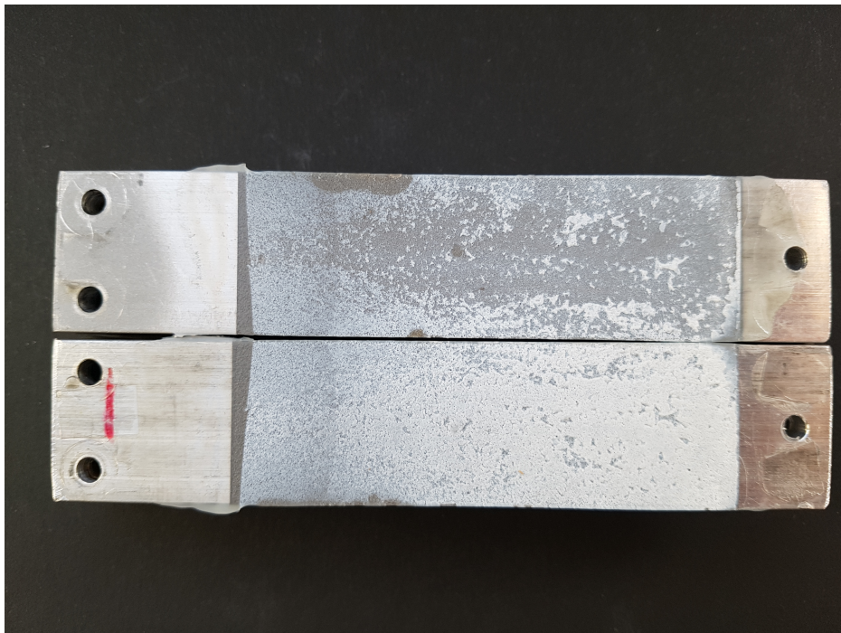
Fig. 5.32 Fracture surface of a fatigue tested T-joint ( ED=5.71 \text{ J/mm}^2 and H=50 \mu\text{m} ) [158]
