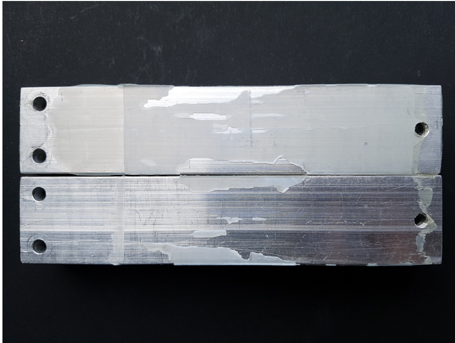
Fig. 5.24 Fracture surface of a fatigue tested degreased joint [158]
