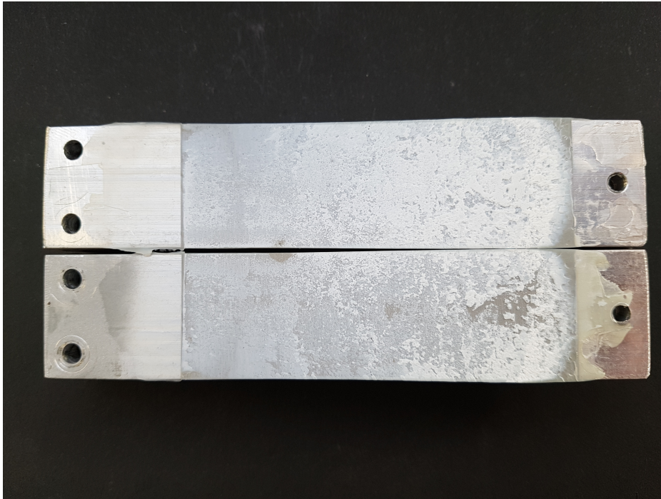
Fig. 5.29 Fracture surface of a fatigue tested T-joint ( ED=1.14 \text{ J/mm}^2 and H=50 \mu\text{m} ) [158]
