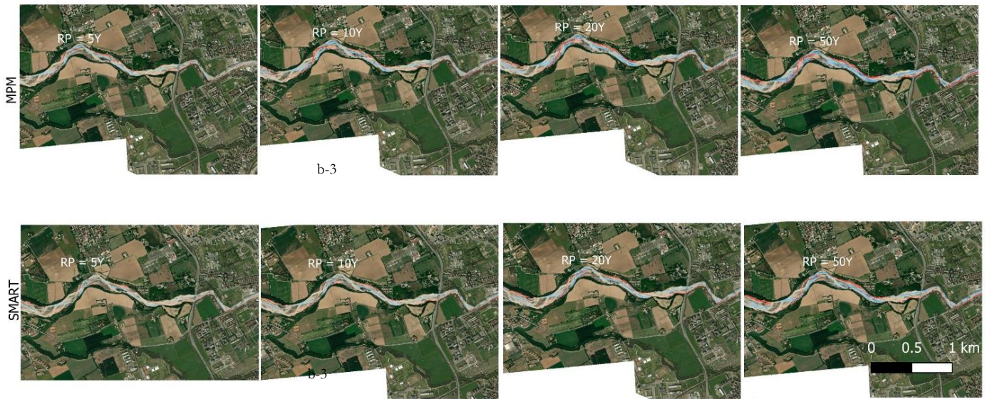
Figure 5.51 Net erosion and deposition progression under different return periods with MPM and SMART approach at location 3.
