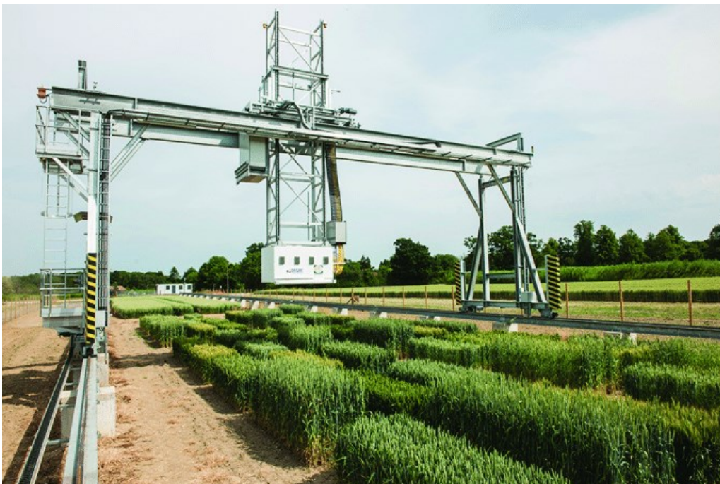
Fig. 8 - A field phenotyping platform consisting of an automated structure moving on two rails. The sensing devices are embedded inside central tower, which is lifted according to crop's height, so that the operation can be conducted fully automatically (Sadeghi-Tehran et al. 2017).
