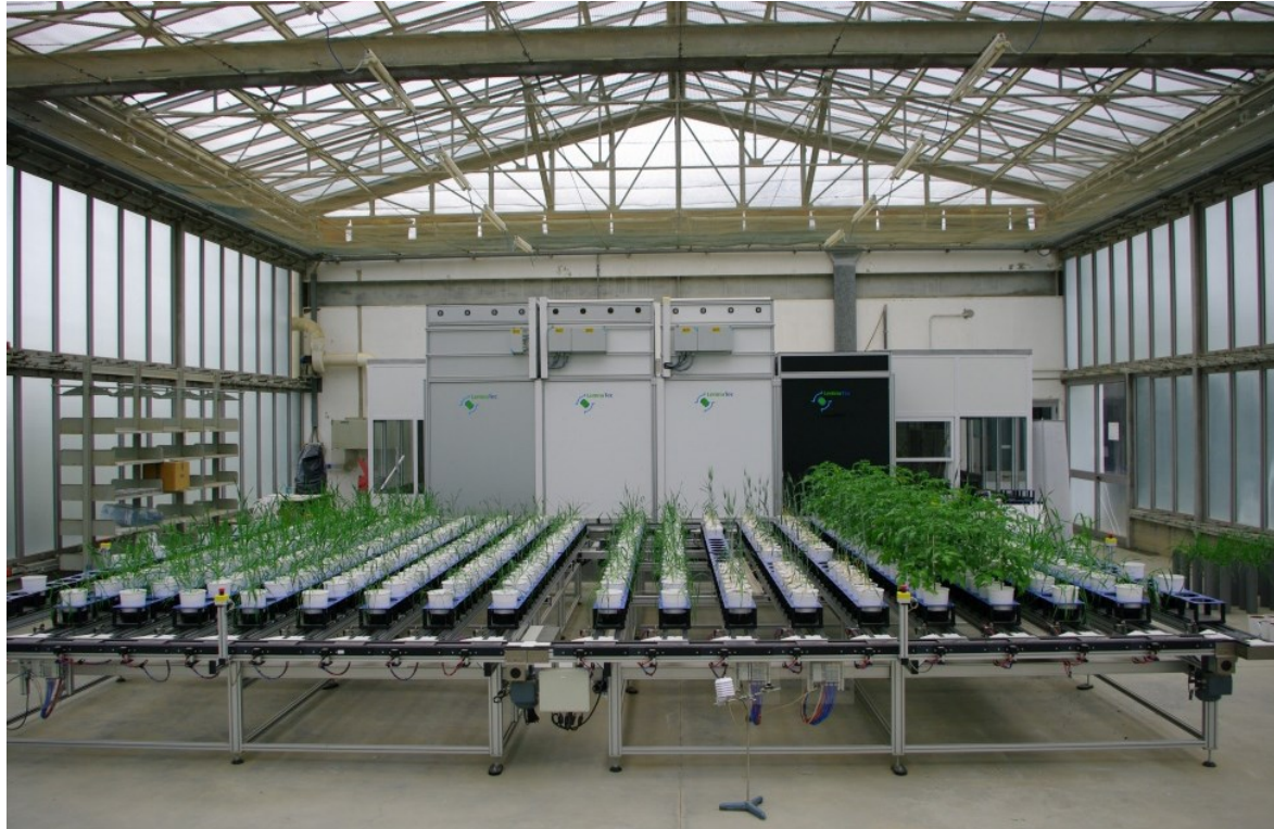
Fig. 53 - High-throughput phenotyping platform, front view. The conveyor with the carts laying upon it is clearly visible in the foreground. The image chambers are the 4 cubic structures in the figure center, the control room is behind them.
