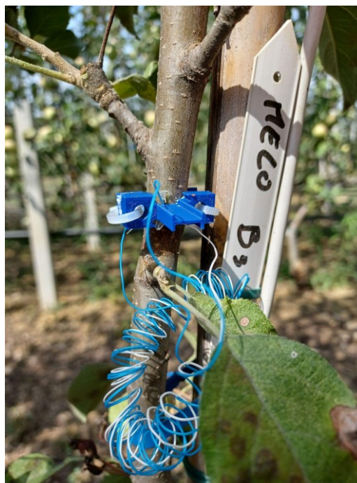
Fig. 21 - Bioristor implementation in Malus domestica . The T-shaped blue part is the holder, fastened around the plant branch. On the right, the sensor's label, use to ease its identification.
