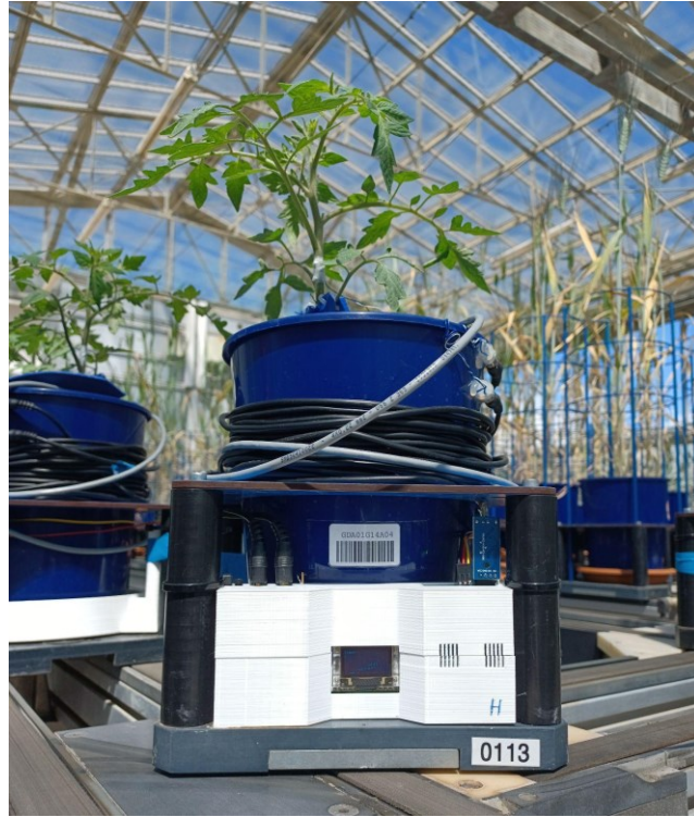
Fig. 58 - Trial of the bioristor control unit in the Scanzalizer platform on tomato plants.
