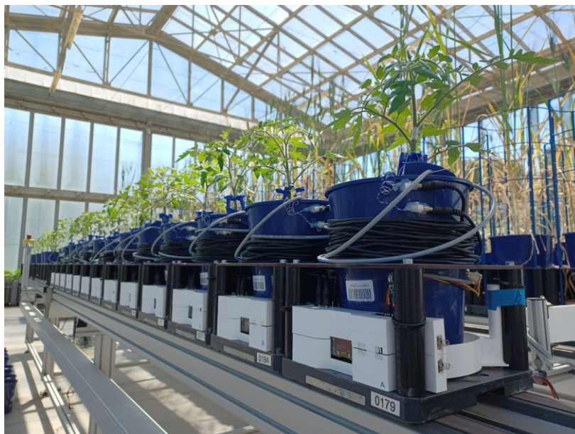
Fig. 59 - Bioristor control unit installed in the Scanzalizer conveyor line.
