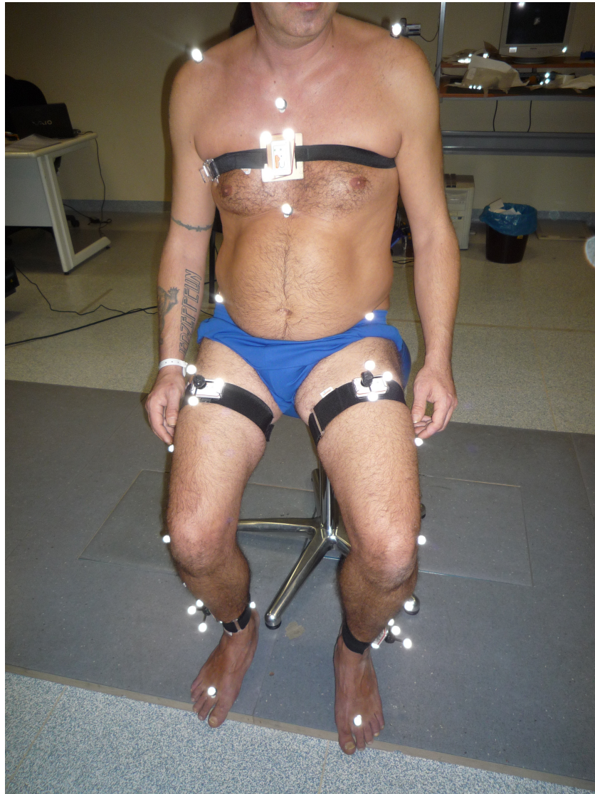
Figure 4.2: Overview of the experimental testbed applied to a monitored subject: both passive markers and Shimmer wireless nodes are considered.
