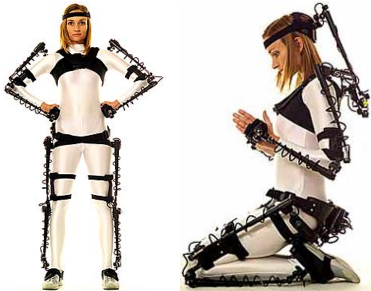
Figure 1.9: Gypsy [5]: a commercial example of a mechanical motion capture system from Meta Motion.
