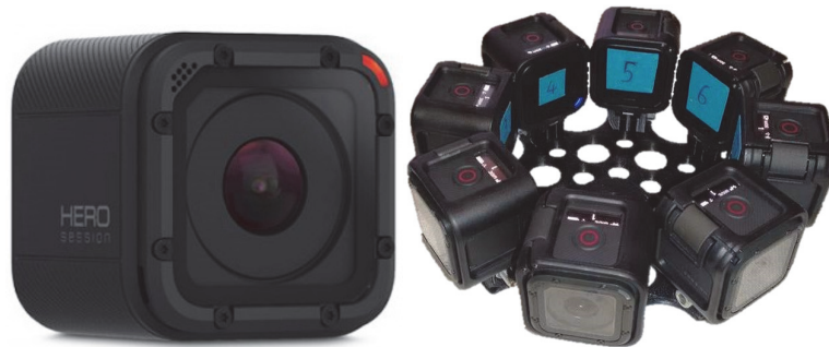
Figure 74: GoPro Hero Session 4 (left) and the prototype of ring for 8 GoPro cameras (right)
