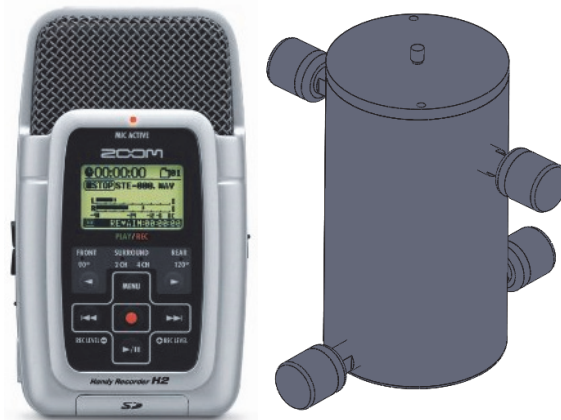
Figure 99: ZOOM H2 (left) and the system assembled for underwater noise monitoring (right)
