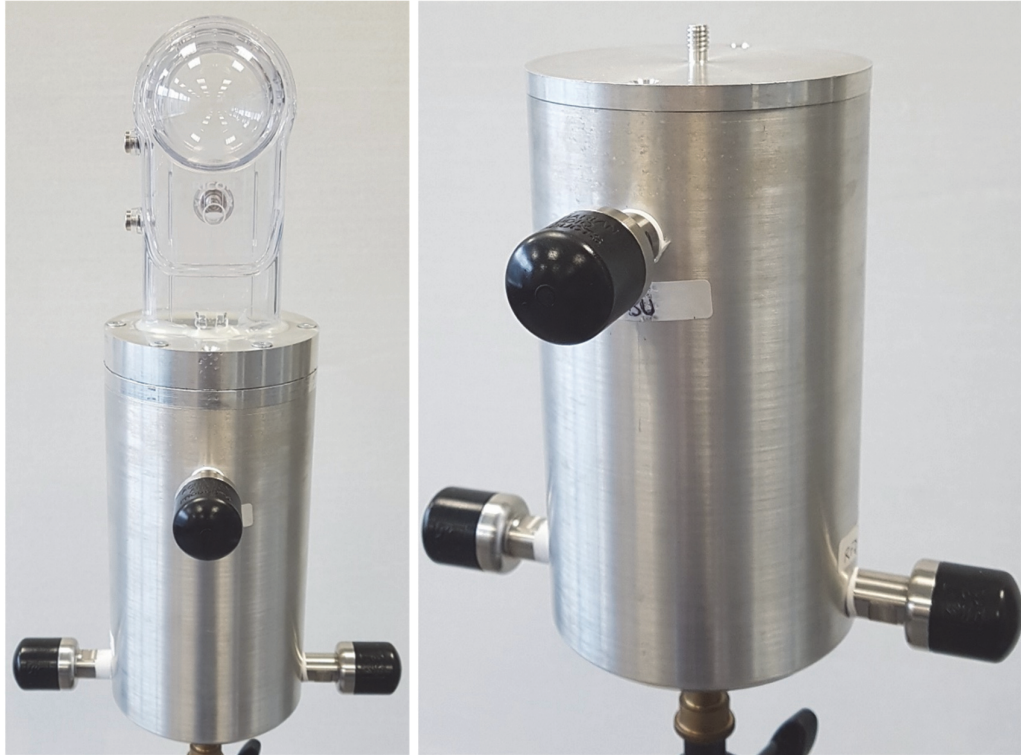
Figure 100: The new underwater array, with panoramic video recording system (left) and with ZOOM H2 recorder (right)
