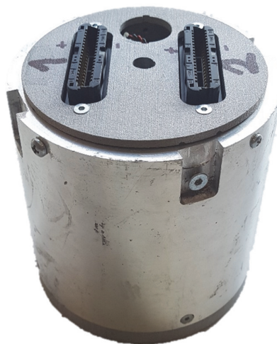
Figure 73: EM electronics for arrays up to 32 channels
