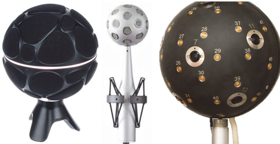
Figure 2: Zylia™ microphone (left), Eigenmike32™ (middle) and Bruel&Kjaer™ array (right)
