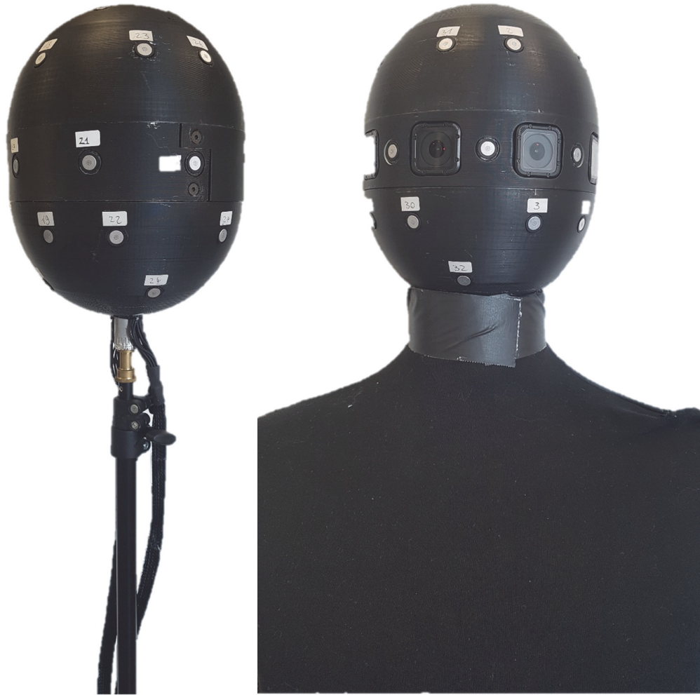
Figure 78: HSA, microphone stand mounting (left) and dummy torso mounting (right)
