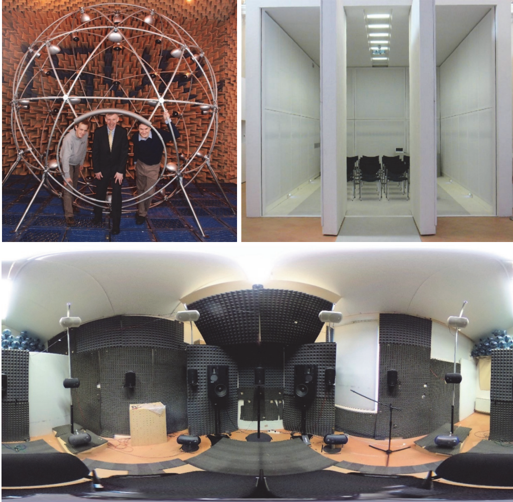
Figure 169: ISVR Ambisonics rig, sphere of 40 loudspeakers (above, left), WFS system in Parma, square of 189 loudspeakers (above, right) and an Ambisonics system in Parma, ring of 8 plus cube of 8 loudspeakers and stereo dipole (below)
