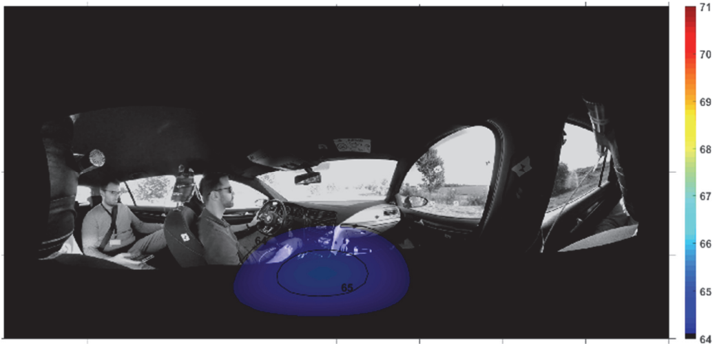
Figure 158: HSA, band-pass filtered map, 70 Hz – 330 Hz, RNC-on
