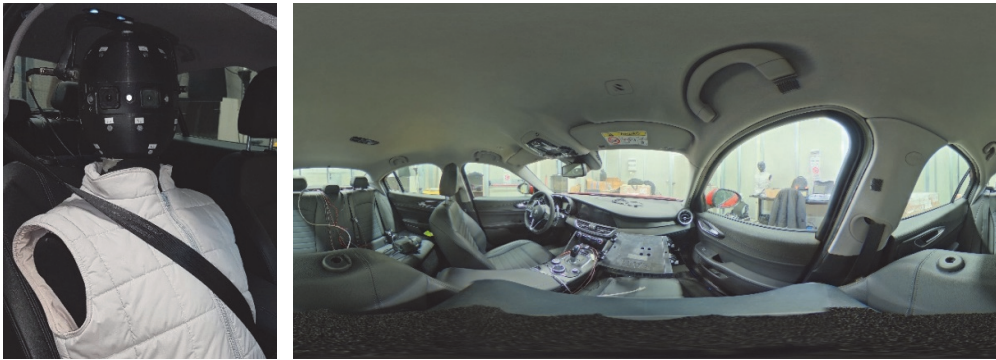
Figure 136: HSA mounted on a dummy torso inside a car (left) and panoramic picture of a cockpit (right)
