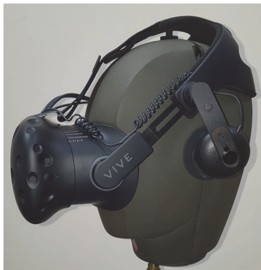
Figure 172: Measurement of the headphones of a HMD with a dummy head
