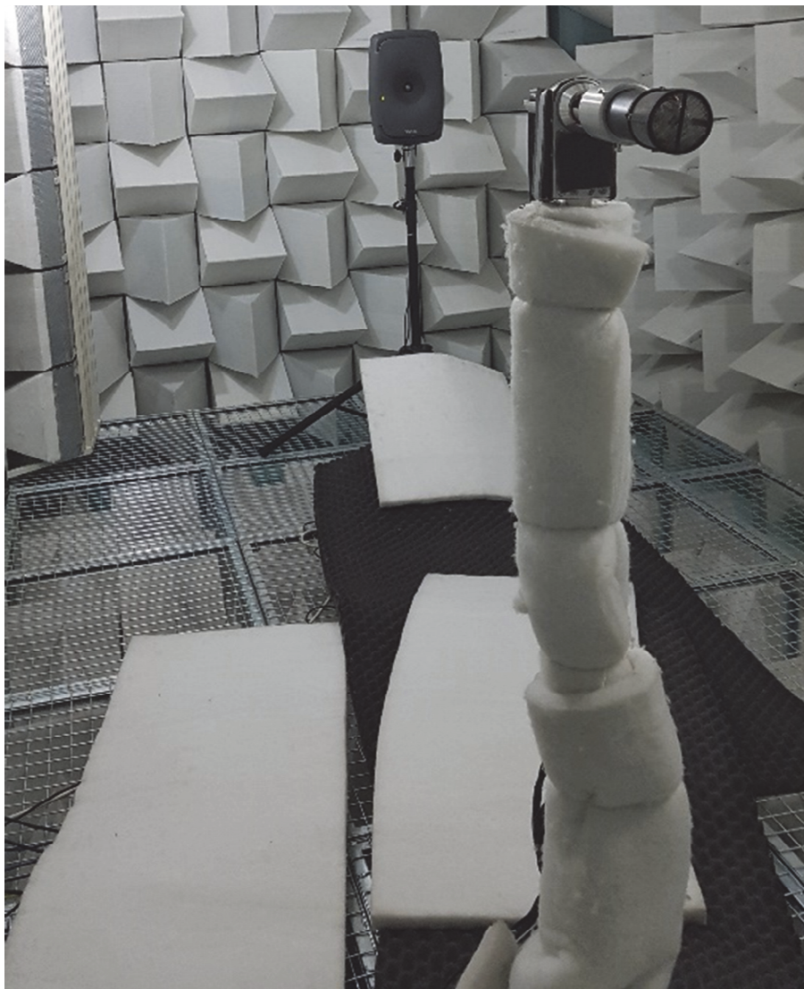
Figure 40: SIR measurement equipment, a two-axis turntable and a studio monitor inside an anechoic room
