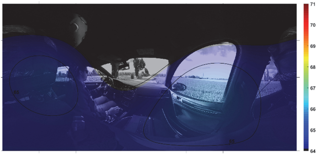
Figure 156: EM, band-pass filtered map, 70 Hz - 330 Hz, RNC-on
