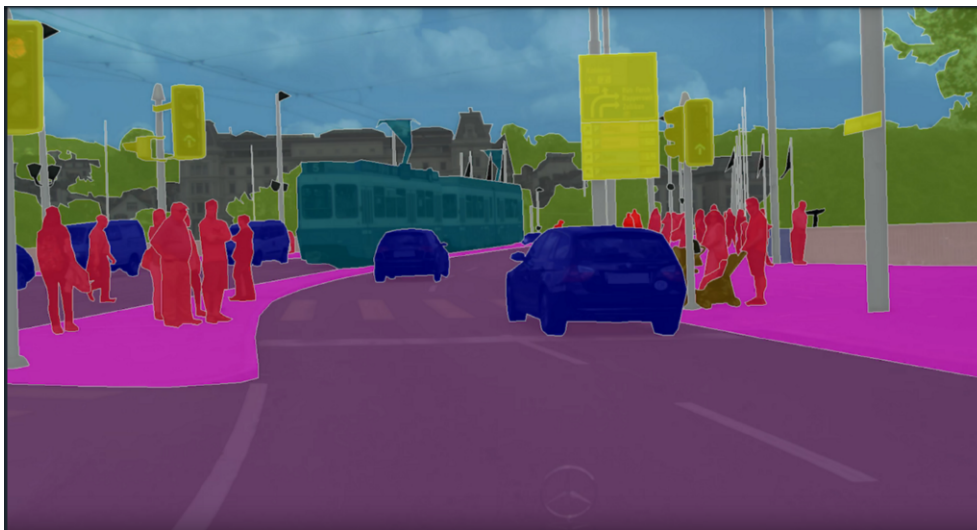
Figure 2.10: Example of semantic segmentation of an image. Each class is assigned a different color for visualization.
