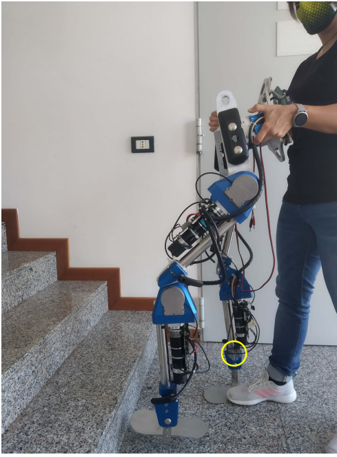
Fig. 3. The experimental exoskeleton used for the tests. A yellow circle points out the ranging sensors positions.
