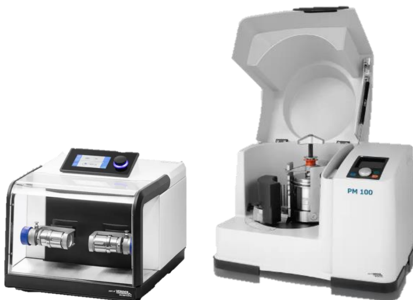
Figure 3.4. Picture of the milling systems adopted during the PhD studies. Left: A Retsch® GmbH (Haan, Germany) mixer-type mill model MM 400, endowed with horizontally oscillatory movements of the reaction jars. Right: A Retsch® GmbH (Haan, Germany) planetary ball mill model PM 100, endowed with 80 mL agate jar and spheres ( \varnothing 15 mm). Pictures taken from Retsch® website ( https://www.retsch.com ).
