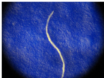
Figure 107. Detail of eraser residue on sample AL_Mi403 (45X).
