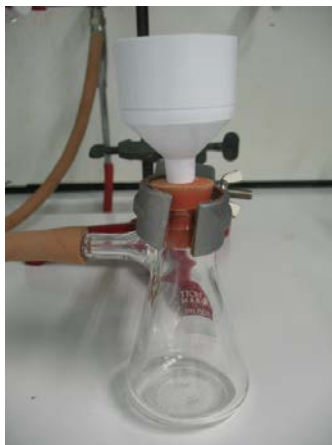
Figure 2. Filtration system consisted of a Büchner filter, a flask and a water pump for the vacuum.
