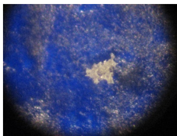
Figure 115. Particular of surface treated with G_Wb_2 characterized by the presence of a fragment of gum (45X).
