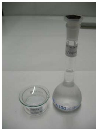
Figure 3. Filtered solution in volumetric flask, separated from the calcium salt powder.
