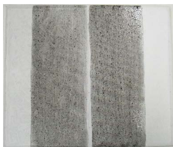
Figure 12. White acrylic drafting sample, with not treated and soiled areas.
