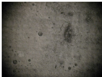
Figure 105. Detail of samples S_KK_tr (7X), cleaned with make-up sponge. We can observe the presence of polymer residues as black particles.
