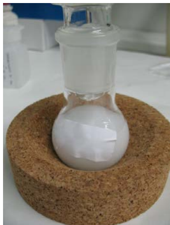
Figure 1. Reaction flask with calcium salt powder and chelating solution.
