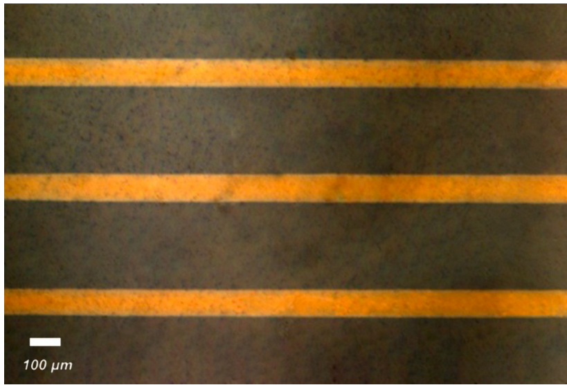
Figure 3.6: Gold electroless stripes deposited by the scanning pipette technique on a CZT sample.
