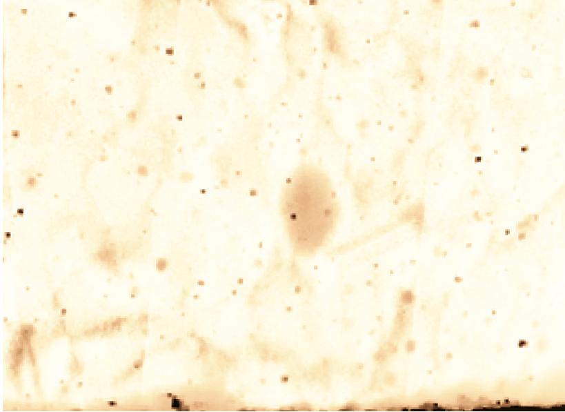
Figure 2.8: X-ray response map of a IMEM sample. Raster scan resolution is 20 \mu\text{m} , beam energy is 25 keV.
