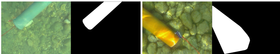
Figure 3.6: Mask generation based on ROI_{area} approach. On right image, an over estimation effect is evident.
