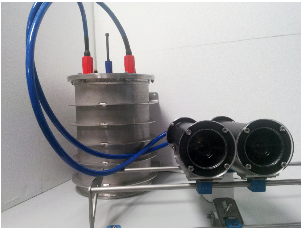
Figure 2.12: Underwater vision system: the vision canister (left) and the stereo rig (right) with the two camera canisters.
