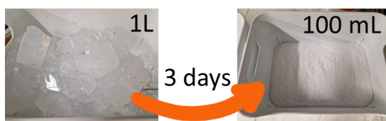
Figure 2.3.5 Batch of sol-gel silica. A considerable reduction in volume can be observed after drying.
