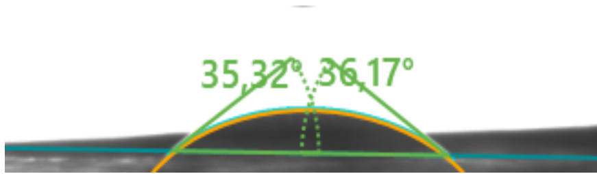
Figure 47- Example of contact angle for the paper coated with the CNC 11 Wt% suspension
