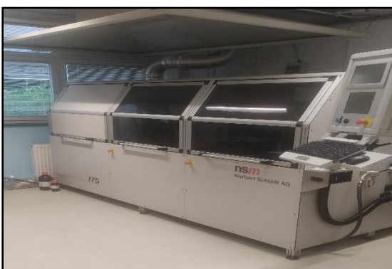
Figure 42- Slot-die coating system of the University of Maribor
