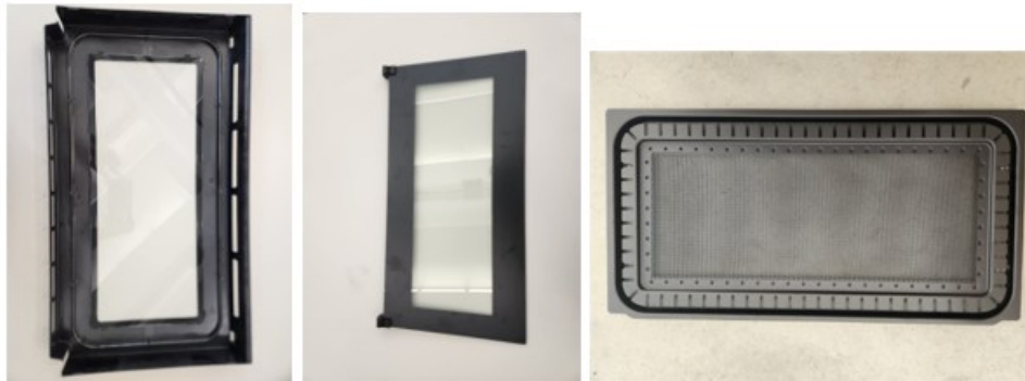
Figure 5.6 Door module disassembly and the main components identified during manual inventory development.
