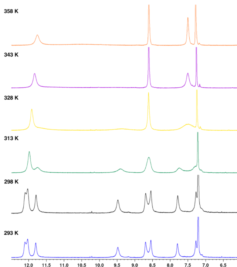
Figure 1.25: ^1\text{H} NMR (600 MHz) spectra of AZ11 in dry \text{DMSO-d}_6 measured at different temperatures.
