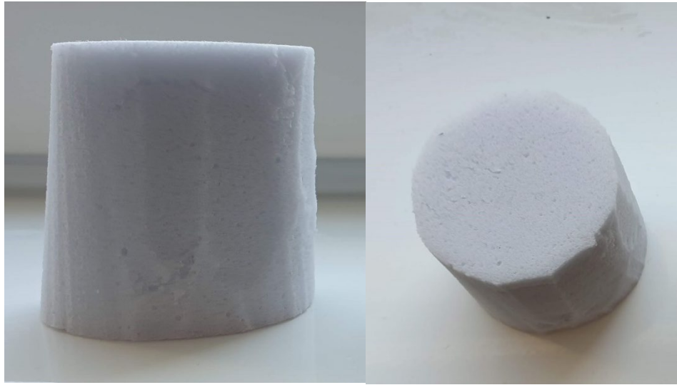
Figure 2: Basotect sample (diameter 4.5cm, height 5cm)
