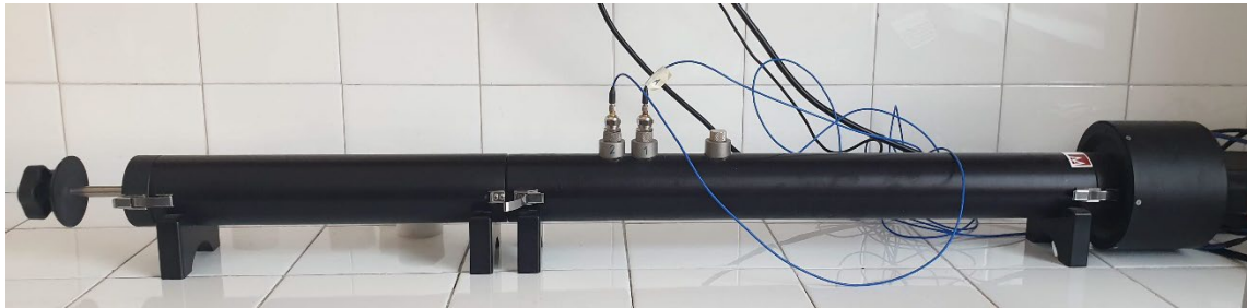
Figure 10: Kundt's tube set up for absorption study with two microphones.
