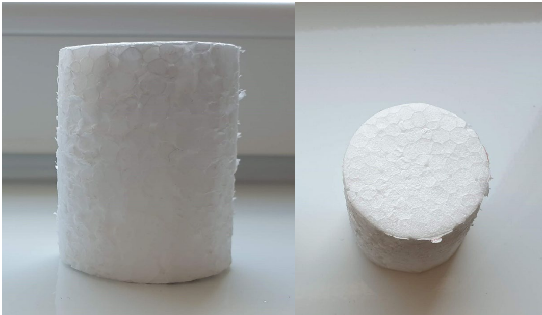
Figure 3: EPS sample (diameter 4.5cm, height 6cm)
