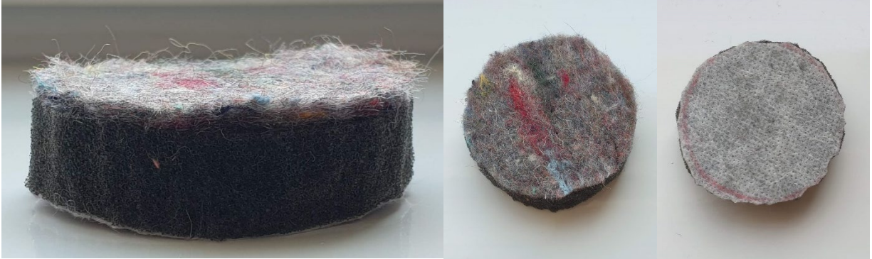
Figure 5: Sample of non-woven fabric (diameter 4.5cm, height 1.4cm), with focus on the right on the two different bases of the same non-woven cylinder.
