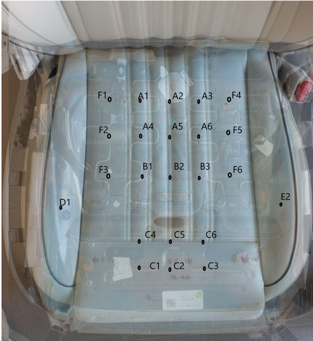
Figure 54: Overlap of top and bottom parts of the seat to show what the sound wave encounters along its path.
