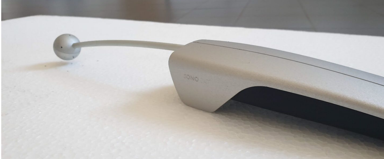
Figure 24: Detail of the SonoCat probe showing how the body of the structure itself maintains a fixed distance between probe and sample.
