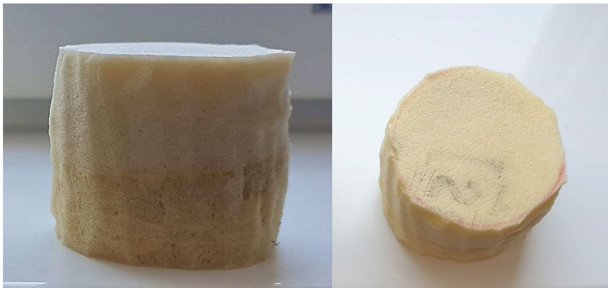
Figure 4: Sample of expanded polyurethane (diameter 4.5cm, height 4.5cm)
