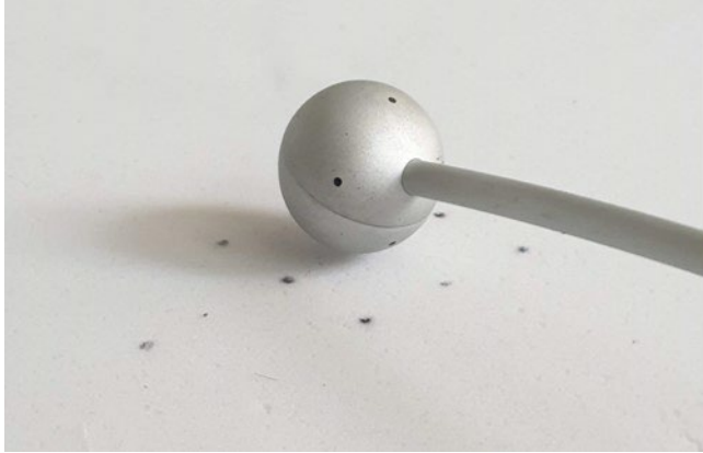
Figure 27: Detail of the probe during measurement of localized points on the sample (schematized on the right) where the double point in the left photo is taken as a reference for mapping point positions relative to the sample.
