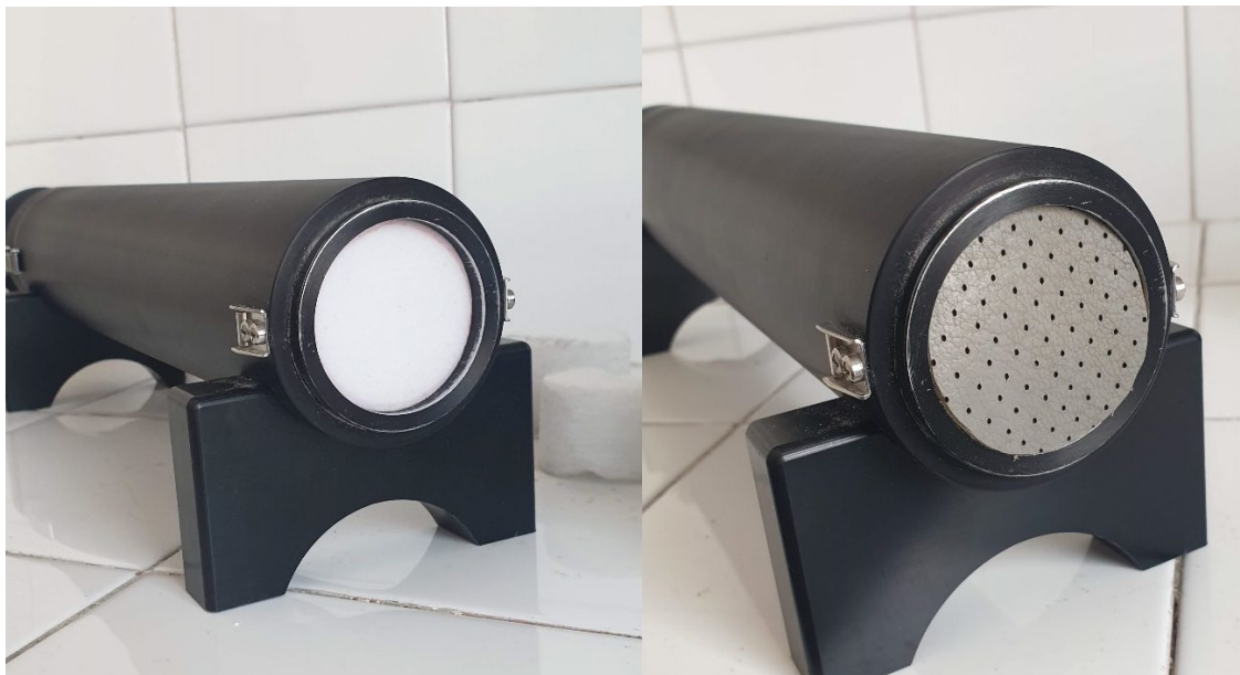
Figure 11: detail of the Kundt's tube in which the calibration sample is placed on the left (melamine) and one of the measured samples on the right (in this case the perforated leather).
