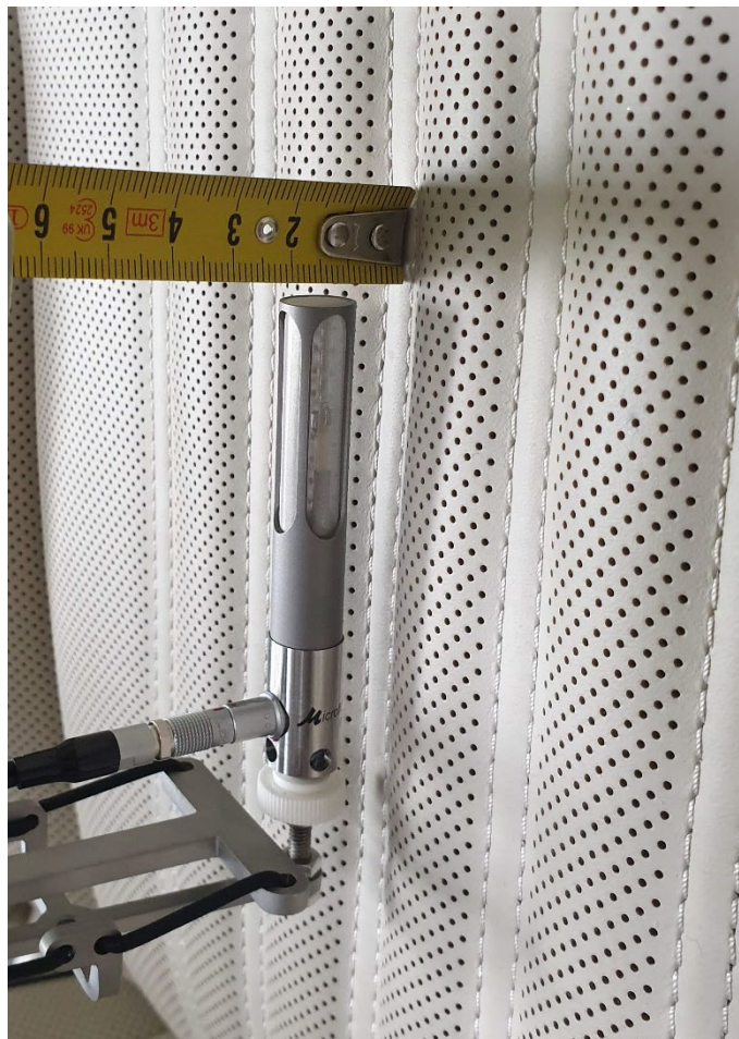
Figure 16: Measurement distance of Microflown probe from sample (in this case the seat backrest).
