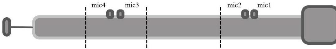
Figure 7: Diagram of the four-microphone Kundt's tube used at the UNITS laboratory (using only 2 microphones).
