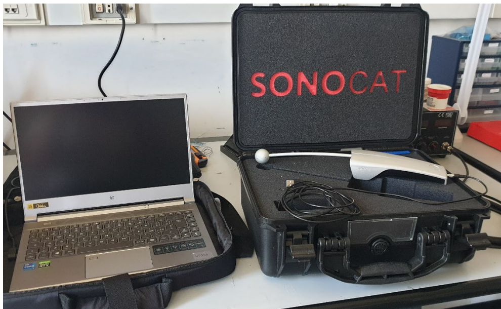
Figure 26: Instrumentation obtained from renting the Sonocat probe, including probe, connection cable, laptop with native software.
