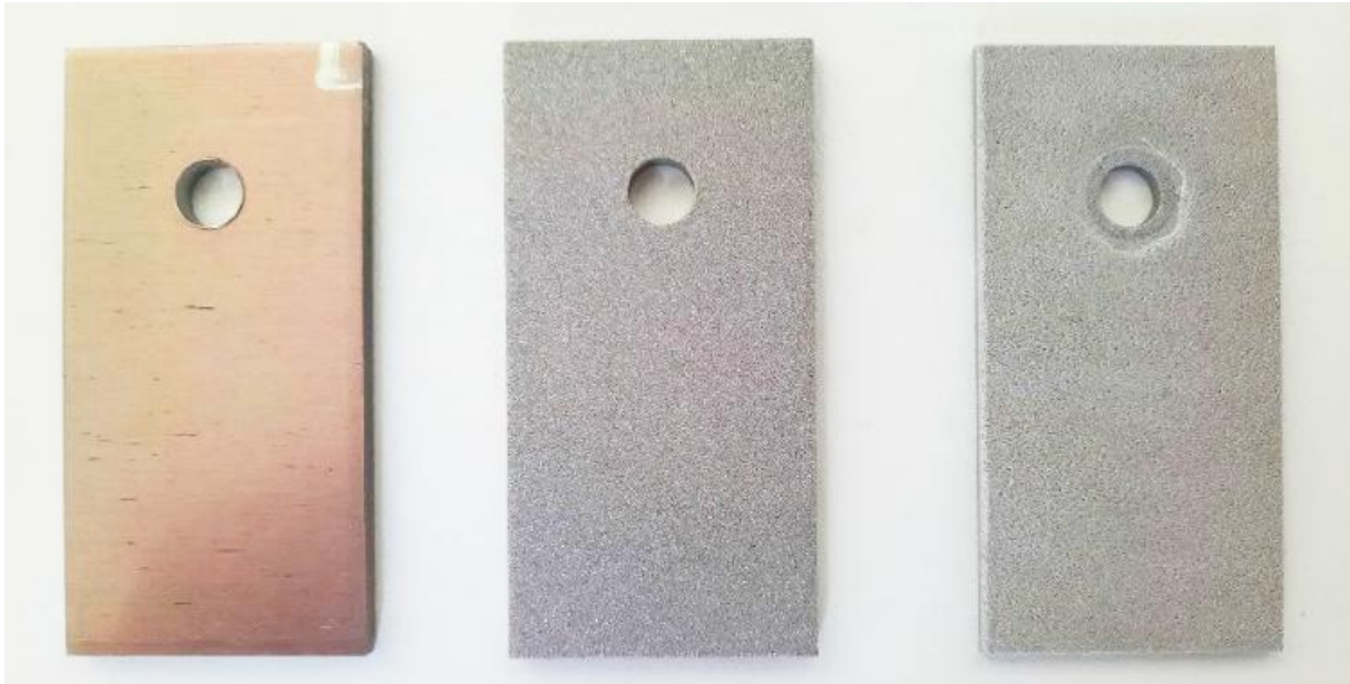
Fig. 100 Left: smooth sample (s); Middle: sandblasted sample (sb); Right: sample prepared by cold spraying (cs).
