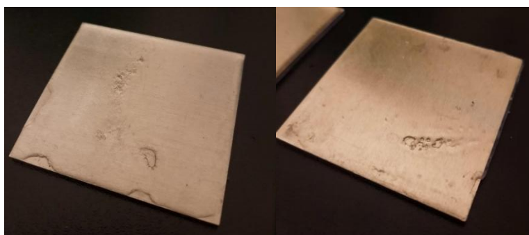
Fig. 62 Sylgard186 samples show non-uniformity of coating with the presence of parts that are not properly cross-linked creating defects. Left Sylgard186 in 1:1 ratio. Right Sylgard186 in 2:1 ratio.
