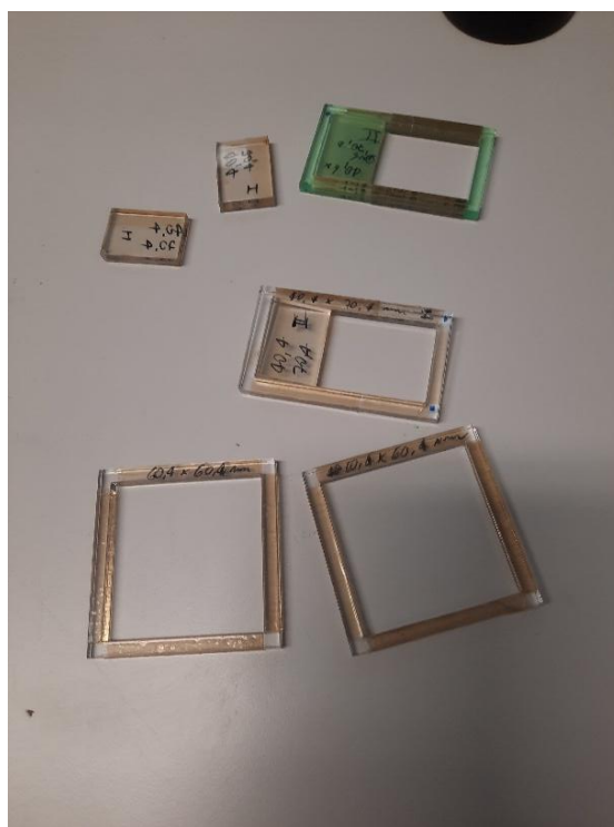
Fig. E1 PMMA moulds in size 30 x 60 x 5mm and 50 x 50 x 5mm. Thanks to Betul Aktas for the molds.
