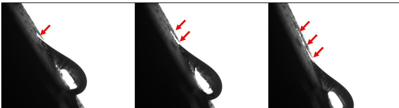
Fig. 46 Droplet pinning on Sylgard184 10:1 surface aged for 30 days. As we can see from the picture, the droplet leaves a path during the movement (red arrows) showing his interlocking on the surface due to dust or impurities present on it.
