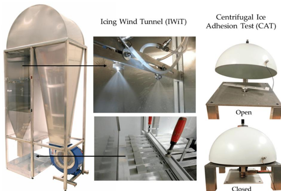
Fig. E2 Left Icing wind tunnel used to create ice on the surface of the samples. At right is the centrifuge used to calculate anti-icing properties through shear stress evaluation 191 . Thanks to Niklas Kandelin and Ruqaya Khammas for help during measurements.
