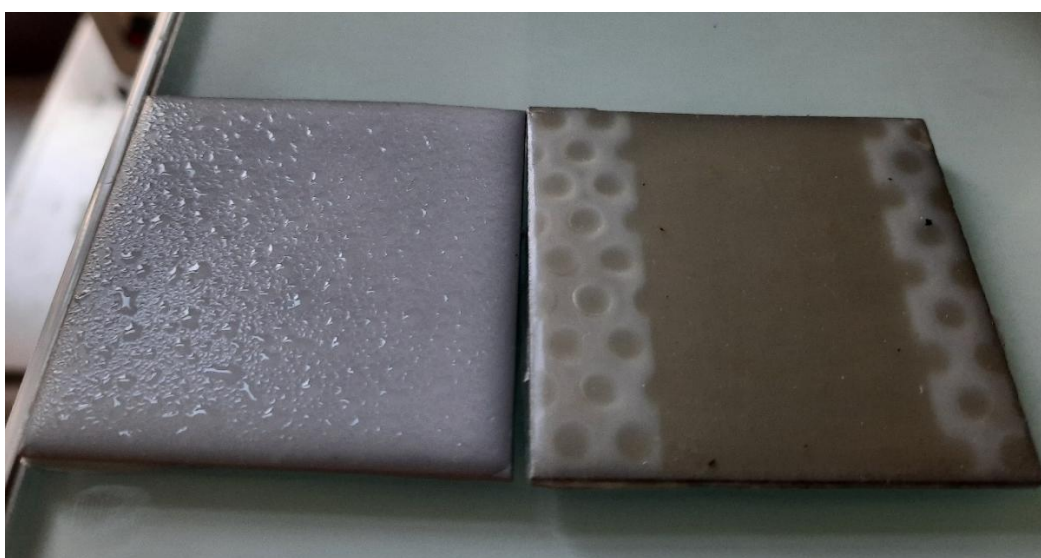
Fig. 86 On the left is the 30:1:6 sample after seven days of maturation at room temperature in the laboratory. On the right is the 30:1:6 sample after the accelerated aging test in a chamber. The latter shows visible signs of degradation caused by the test.
