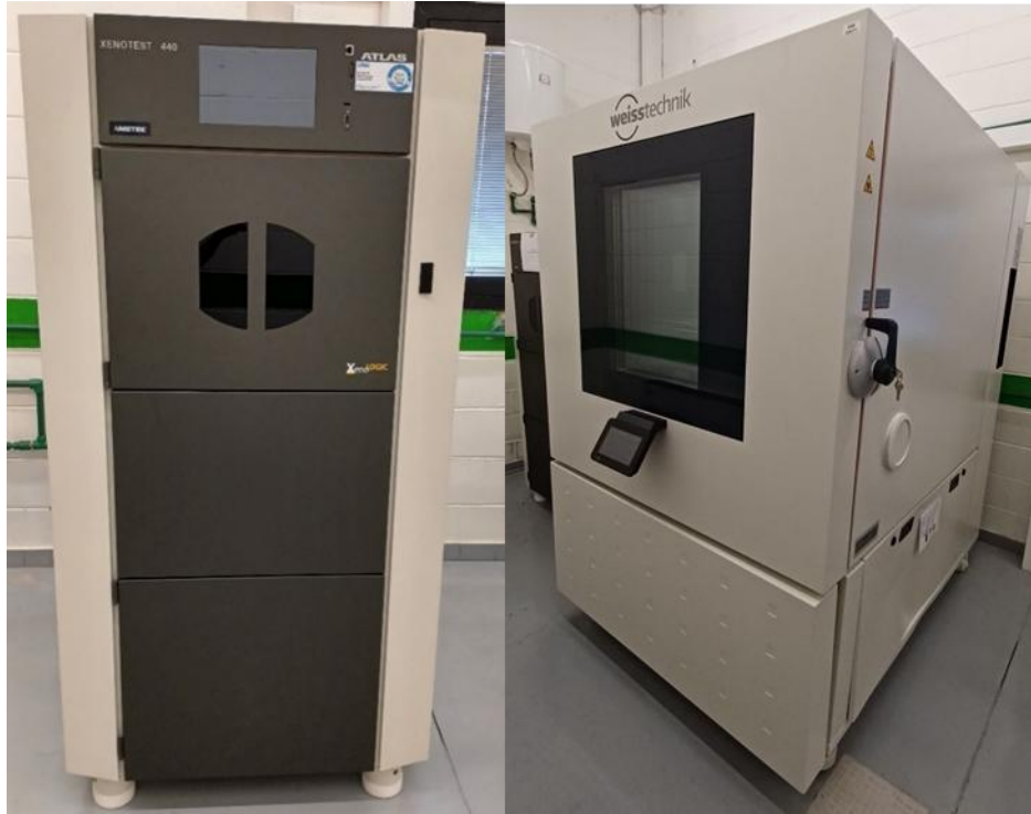
Fig. E3 On the left Atlas® Xenotest 440 climate weathering test chamber. On the right Weiss Technik® ClimeEco C7.1000 climate chamber. Thanks to Paolo Gadia for the tests.
