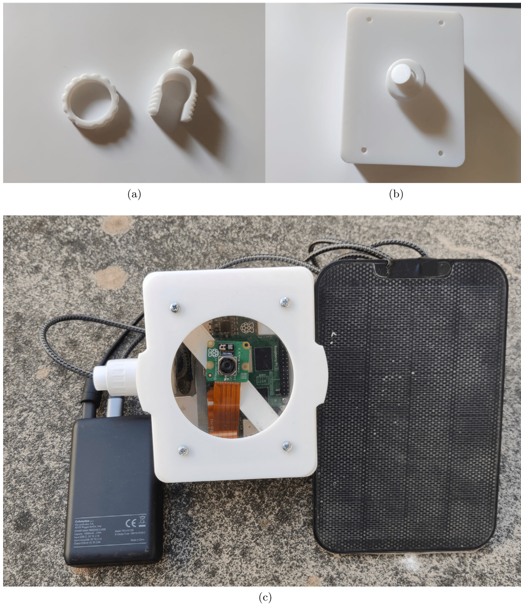
Fig. 9. Pictures of the ANTPi components: (a), and (b) show the 3D-printed case sub-components from different perspectives; and (c) shows the whole hardware system along with the solar panel and the powerbank.
