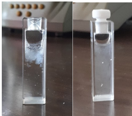
Figure 22. Examples of turbid collagen solutions: the collagen self-assembly increases the turbidity of solution.
