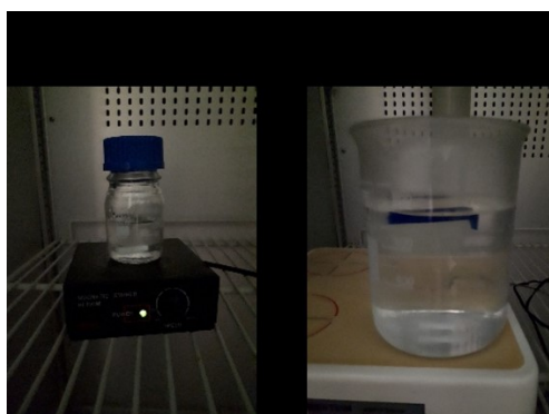
Figure 29. The first two steps of sample preparation protocol. a) Dissolution of collagen in acetic acid, b) dialysis of solution against phosphate buffer.
