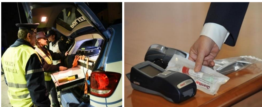
Figure 5.8 Quantisal™ Oral Fluid Collection Device and Alere DDS2 mobile test system used by the State Police
