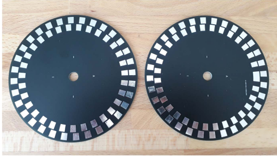
Fig. 7. Photograph of the Vernier disks used for the experimental tests: full-Vernier on the left and half-Vernier on the right. Both have N = 32 . The diameter of the disks is 116 mm.
